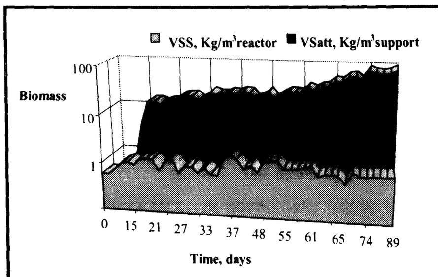
Fig. 3. Profiles of effluent volatile suspended solids (kg VSS/m<sup>3</sup> digester) and volatile attached solids (kg VSatt/m<sup>3</sup> SIRAN) during the colonisation process.
