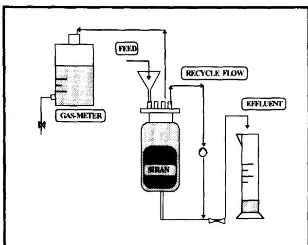
Fig. 1. Schematic diagram of the experimental reactor.
