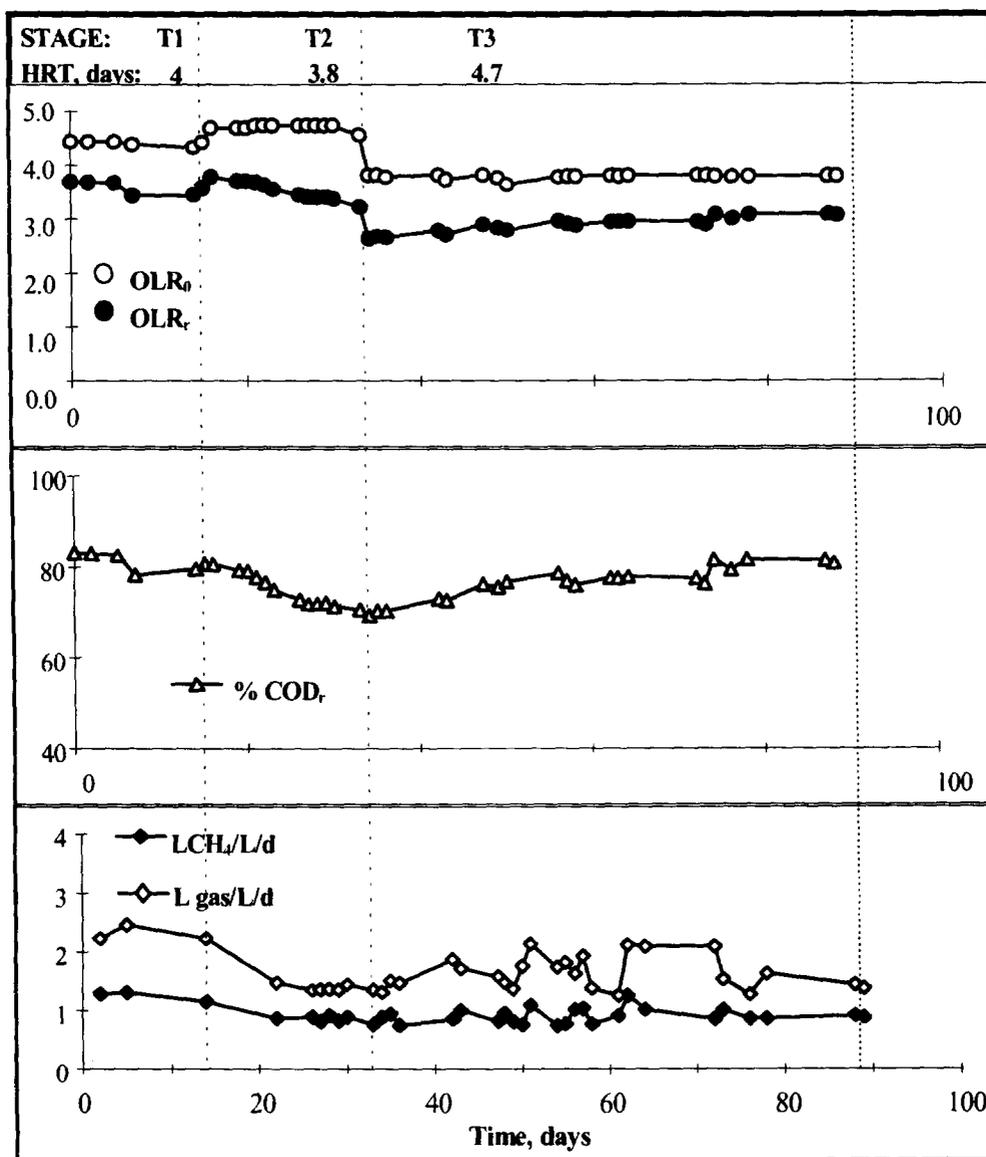
Fig. 2. Variations of the characteristic parameters of the anaerobic process: (a) organic loading and removal rate, OLR<sub>0</sub> and OLR<sub>r</sub>, as kg COD/m<sup>3</sup>/day; (b) COD<sub>r</sub>, organic removal efficiency (as a percentage of initial COD); (c) volumetric CH<sub>4</sub> and biogas production rate, l/l digester/day. Feed: diluted vinasses 18 g COD/l.
