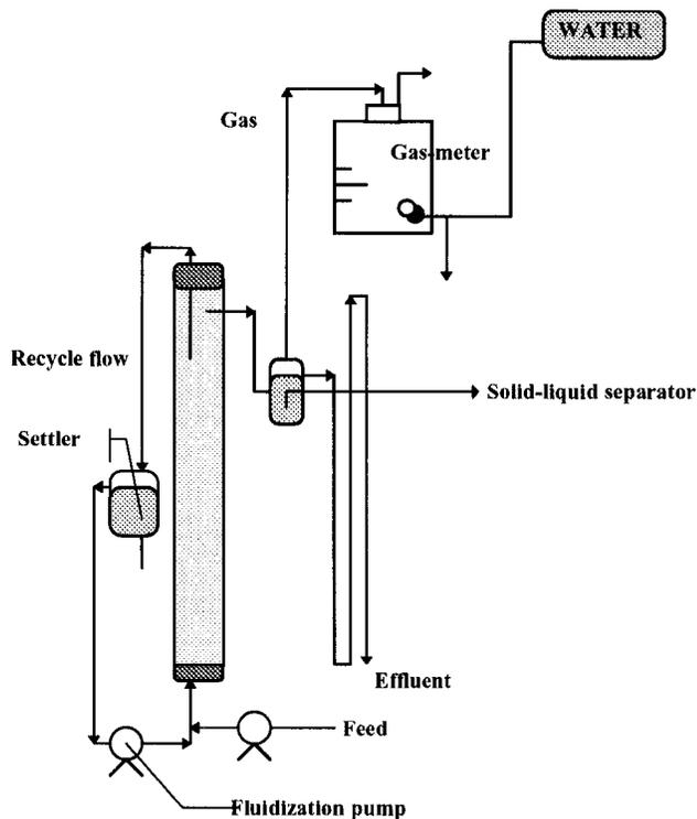
**Figure 1.** Schematic diagram of the experimental anaerobic fluidized bed (AFB) reactor.
