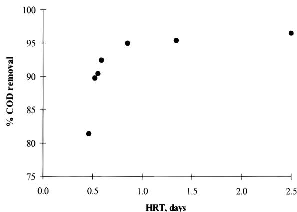
**Figure 2.** Organic removal efficiency (as percentage of chemical organic demand, %COD removal) as influenced by hydraulic retention time (HRT).
