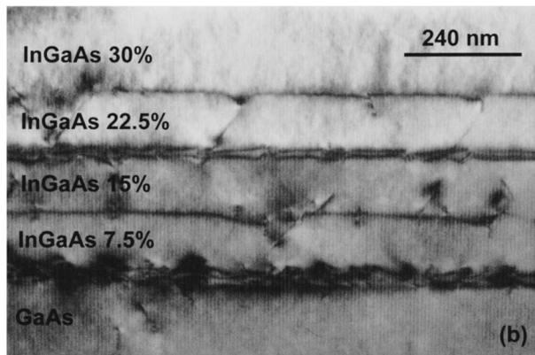
FIG. 2. (a) Bright field g004 XTEM micrographs of sample B; (b) Bright field g004 XTEM micrographs of sample C. Nearly constant MD densities around  $1 \times 10^5 \text{ cm}^{-1}$  and  $1.6 \times 10^5 \text{ cm}^{-1}$  are measured at buried interfaces for samples B and C, respectively. The sample structures are described at the left side of the micrographs. The layer thickness, as for all the samples studied, is 120 nm. Note that no dislocation threads across the structure.
