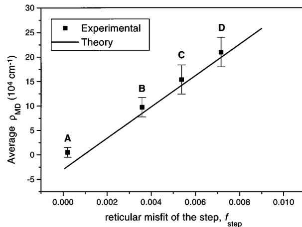
FIG. 3. Average misfit dislocation densities for each structure determined by statistical counting of cross-section TEM observations (open circle with statistical error bars). The predicted work-hardening density (full line) vs the steps of composition are shown to fit very well with the experimental data and can be analytically expressed by the Eq. (3) linear regression of the calculated data.
