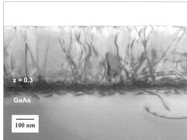
Fig. 3. Cross section micrograph (BF) with  $g0\bar{2}2$  of sample D. The beam direction is  $[0\bar{1}1]$ .
