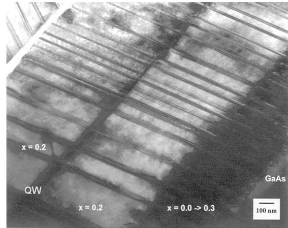
Fig. 5. Cross section micrograph (BF) from sample C with  $g\bar{0}22$ . The beam direction is  $[0\bar{1}1]$ . We can observe an increase in the twin density but no MD are present.
