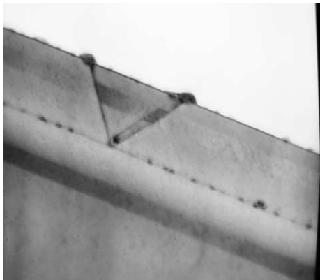
Fig. 2. Dark field (200) TEM cross-sectional images of stacking faults originated from dislocated QDs in samples A1 and A2.
