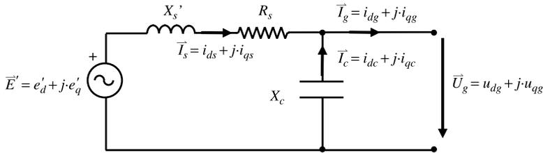
Fig. 3. Equivalent circuit of fixed speed wind turbines.
