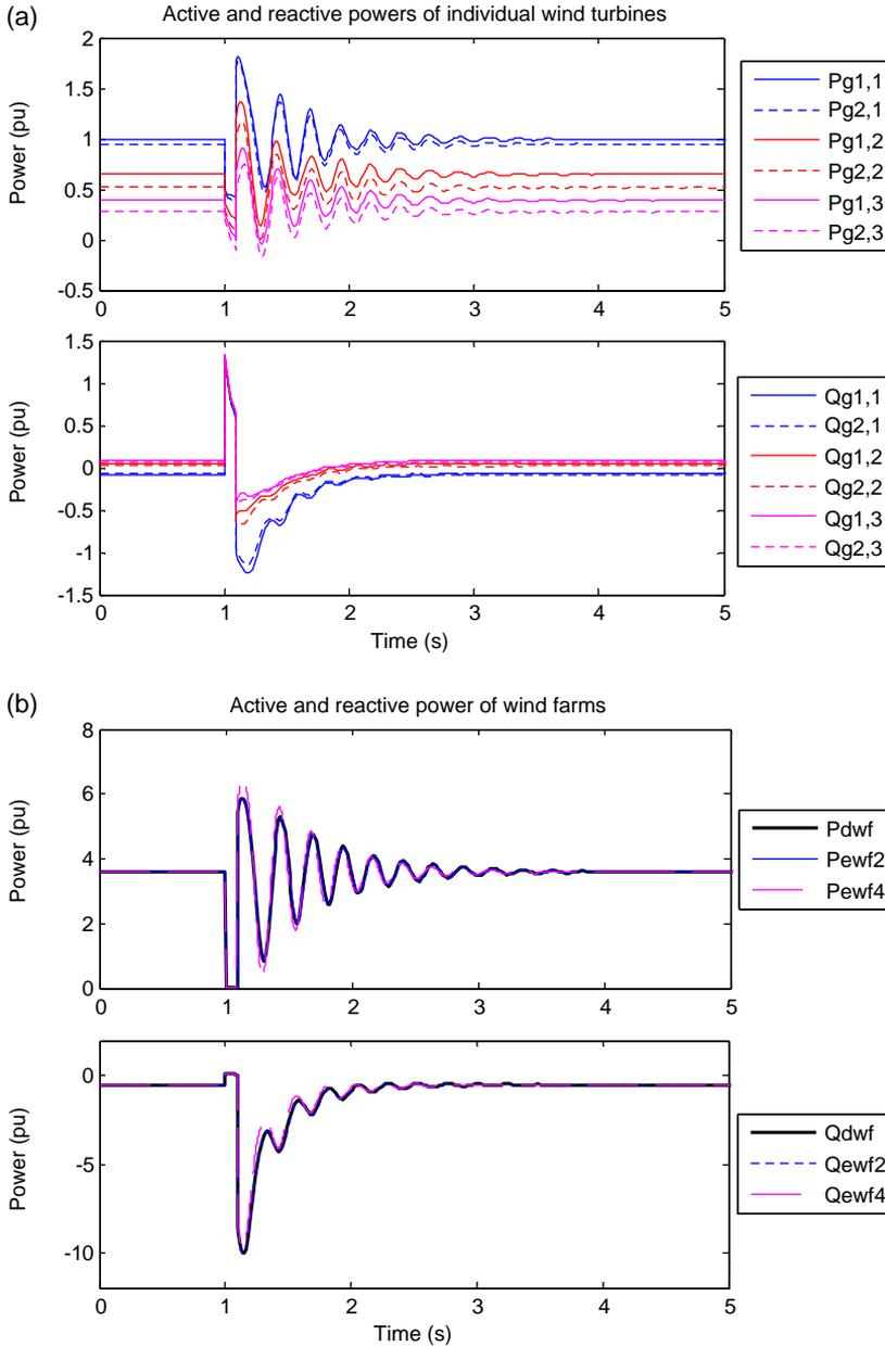
Fig. 20. Simulation results of complete and equivalent wind farms under a short circuit at PCC.
