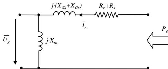
Fig. 8. Steady state induction generator model.
