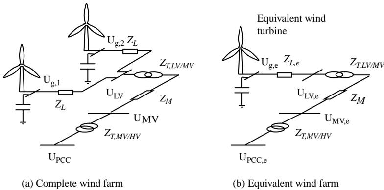
Fig. 11. Complete and equivalent wind farms for steady-state simulations.
