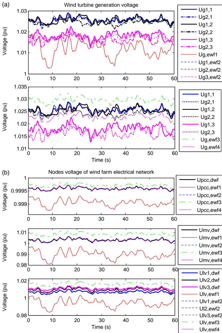
Fig. 19. Nodes voltage of wind farm electrical network for complete and equivalent wind farms with pitch regulated wind turbines under wind fluctuations.
