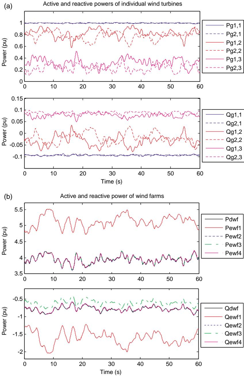
Fig. 18. Active and reactive powers both of wind turbines and wind farm for complete and equivalent wind farms with pitch regulated wind turbines under wind fluctuations.
