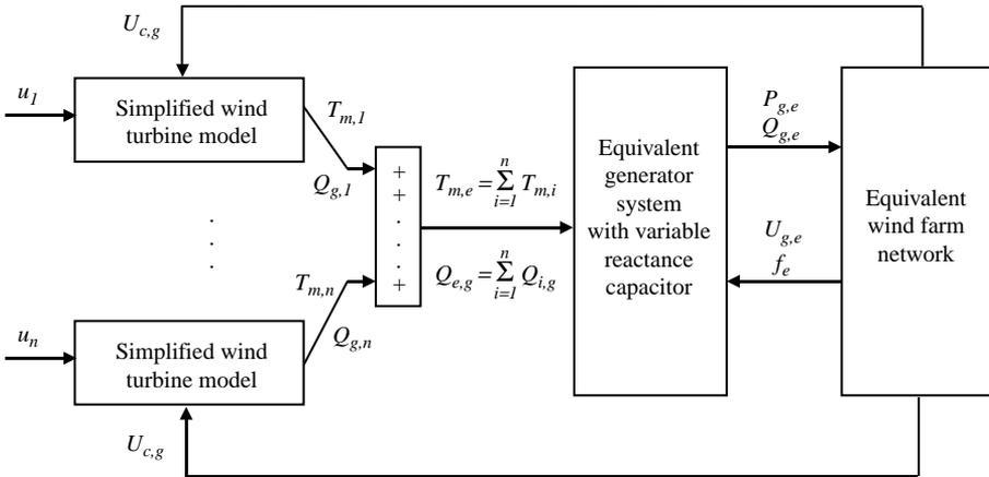
Fig. 9. Equivalent wind turbine with simplified model of each individual wind turbine.
