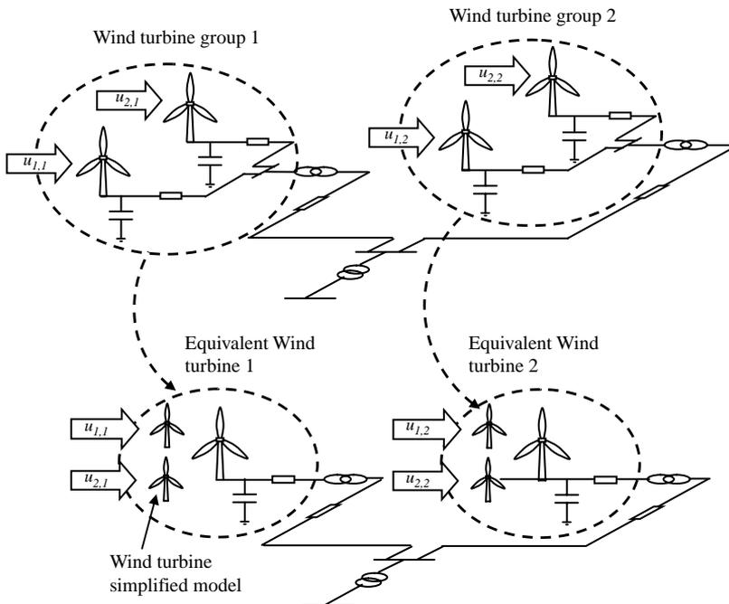
Fig. 7. Equivalent wind farm by using equivalent wind turbines for aggregated wind turbines under different incoming winds.
