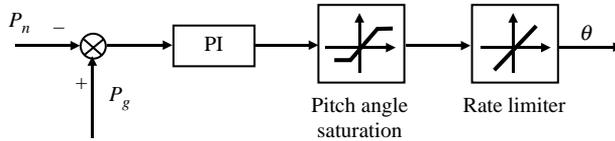
Fig. 4. Control scheme of pitch regulated wind turbines.
