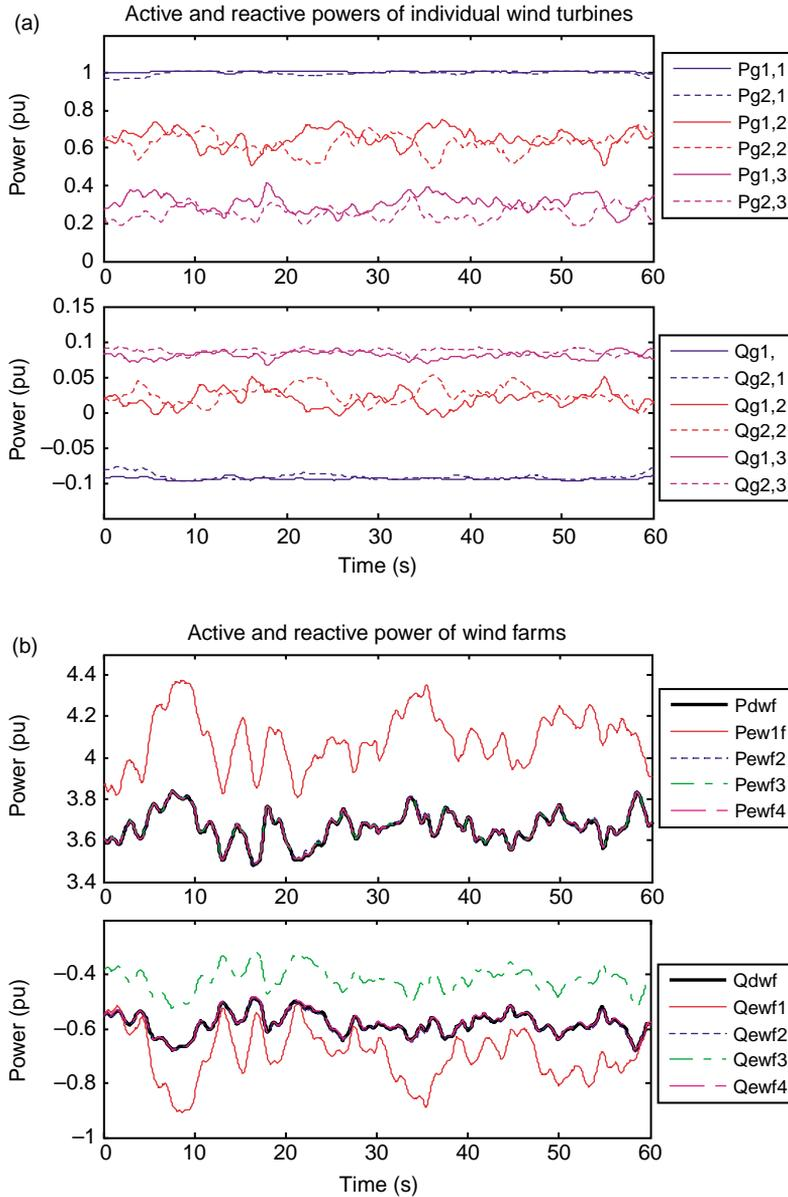
Fig. 16. Active and reactive powers both of wind turbines and wind farm for complete and equivalent wind farms with stall regulated wind turbines under wind fluctuations.
