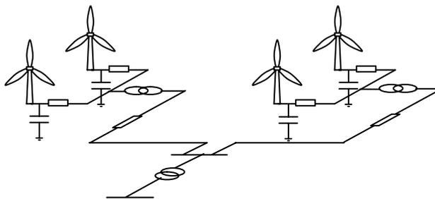
Fig. 1. Wind farm with fixed speed wind turbines.
