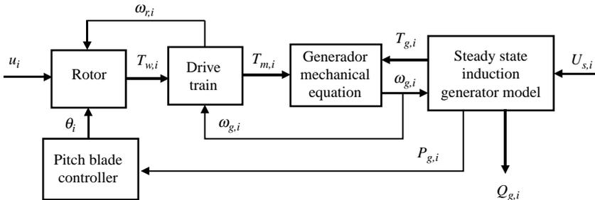
Fig. 10. Simplified wind turbine model.
