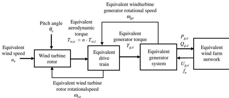
Fig. 6. Equivalent wind turbine model with equivalent incoming wind.
