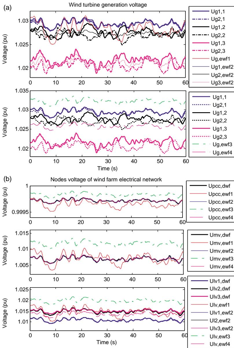
Fig. 17. Nodes voltage of wind farm electrical network for complete and equivalent wind farms with stall regulated wind turbines under wind fluctuations.
