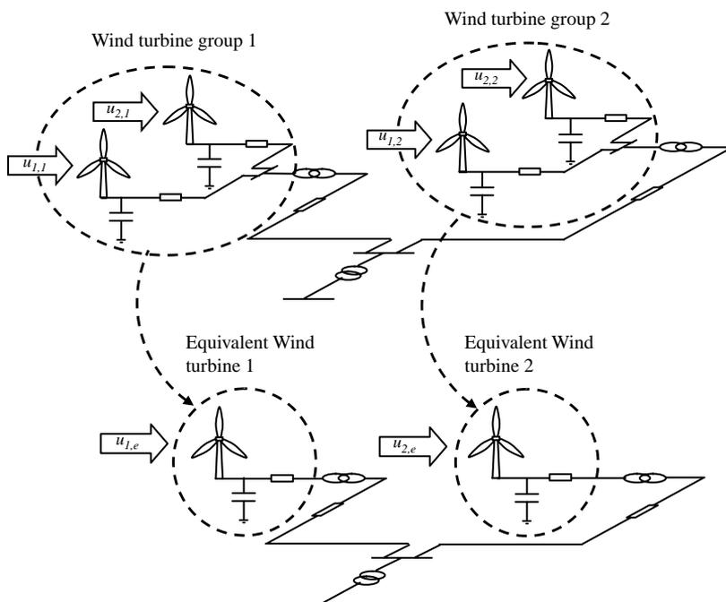
Fig. 5. Equivalent wind farm by using equivalent wind turbines for aggregated wind turbines with similar winds.
