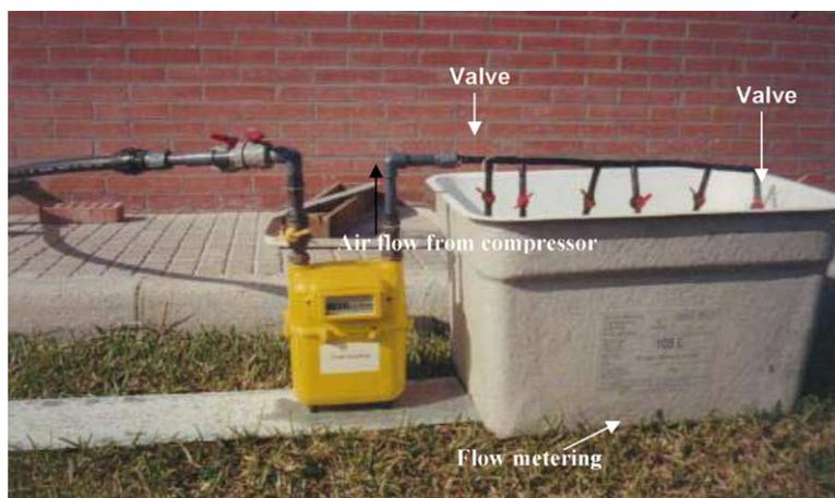
Fig. 1. Batch reactor system used during the experiment.
