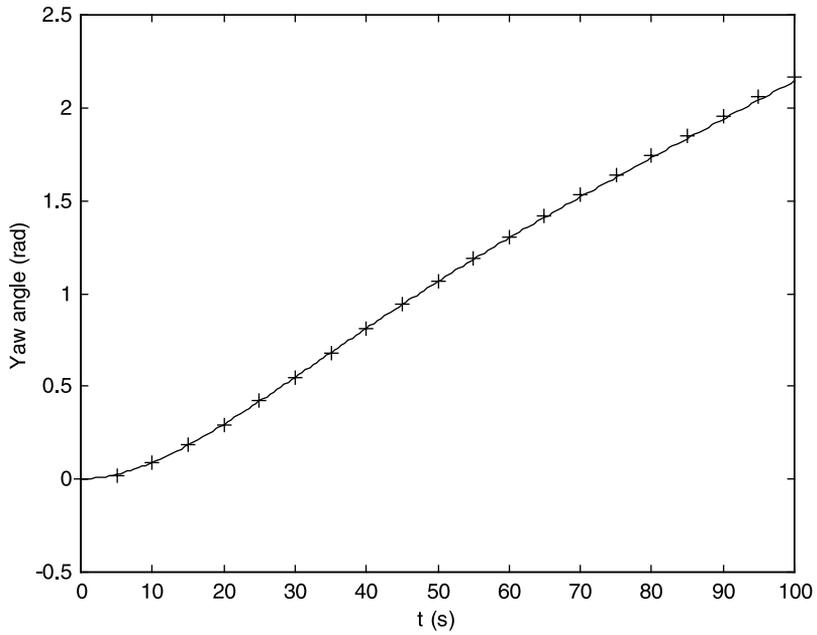
Fig. 3. Time response of the yaw angle. Sign+line: experimental values. Continuous line: polynomial fit.
