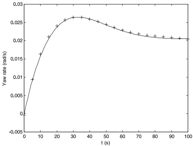
Fig. 4. Time response of the yaw rate. Sign+line: experimental values. Continuous line: polynomial fit.
