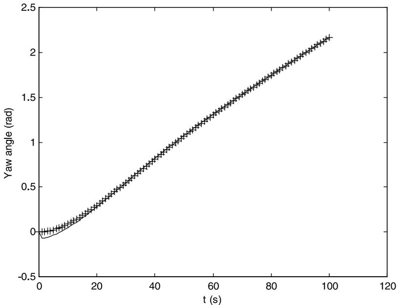
Fig. 8. Variation of the yaw angle. Continuous line: fitted curve to experimental. Data using the least square method. Sign plus: using the parameters identified.
