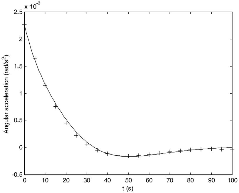
Fig. 5. Time response of the angular acceleration. Sign + line: experimental values. Continuous line: polynomial fit.
