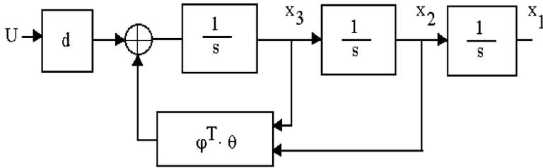
Fig. 6. Block diagram of a third-order parametric strict—feedback analysed system.
