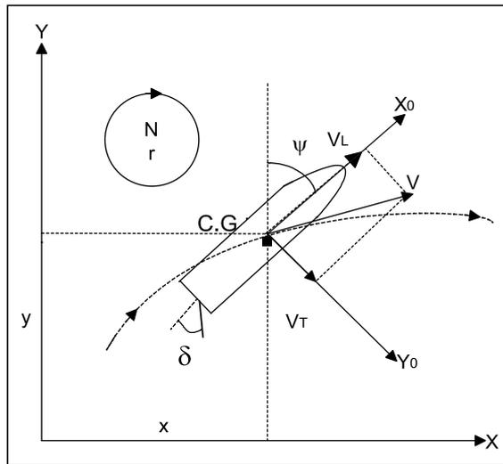
Fig. 1. Co-ordinate systems for the description of ship motion.
