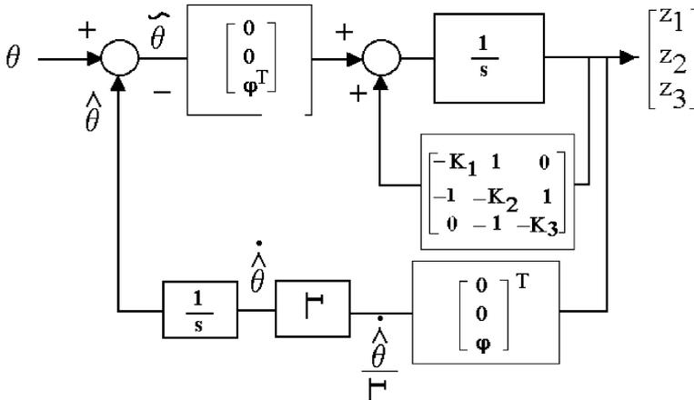
Fig. 7. Block diagram for vector of parameters updating.
