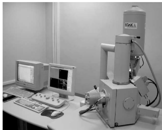
Fig. 3. SEM and EDS equipments used in the experimental stage of this work.
