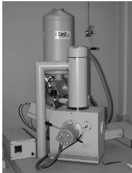
Fig. 4. Scanning electron microscope, Quanta 200.
