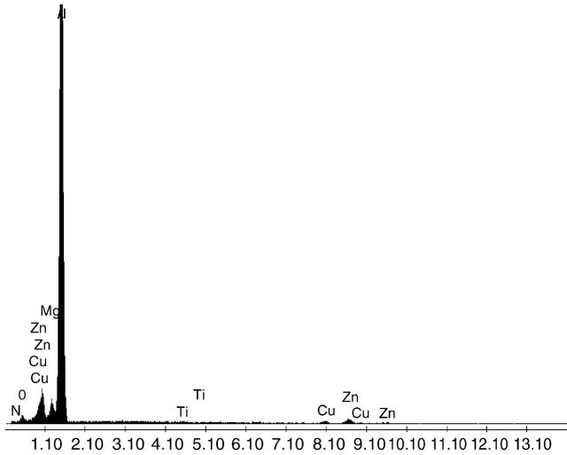
Fig. 9. Energy Dispersive Spectrometer analysis of the tool edge used at  $v = 0.72$  m/s,  $a = 0.05$  mm/rev and  $d = 2$  mm.
