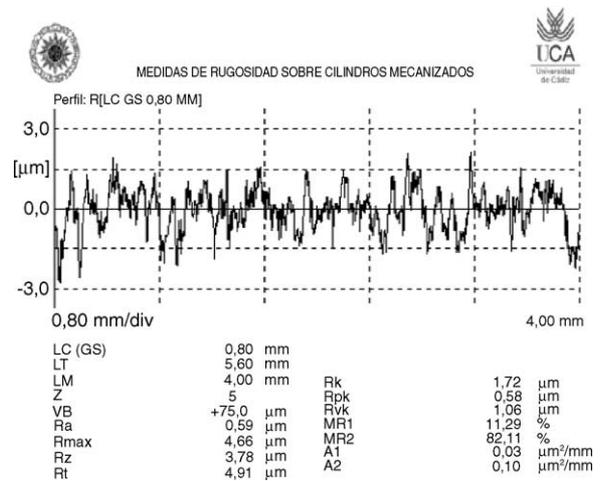
Fig. 3. Protocol for roughness measurement.
