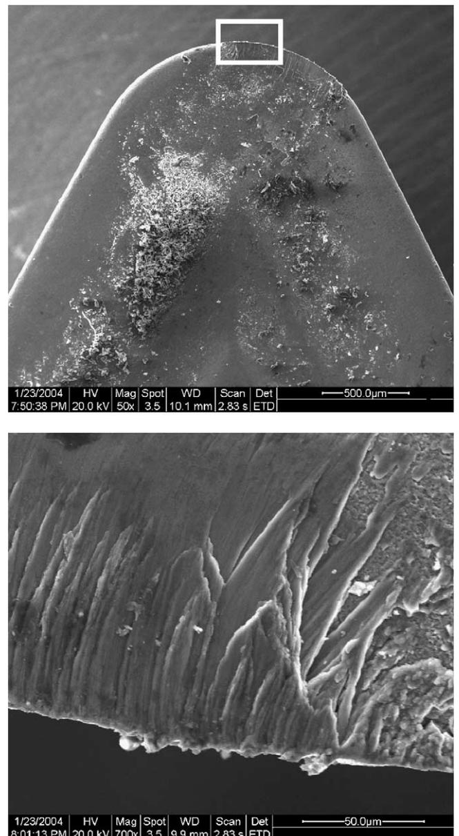
Fig. 8. (a) Adhesion effects on the tool. (b) Edge detail.
