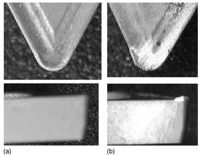
Fig. 11. Tools macrographs used during the machining process of: (a) AA7050; (b) AA2024, under the same cutting conditions.
