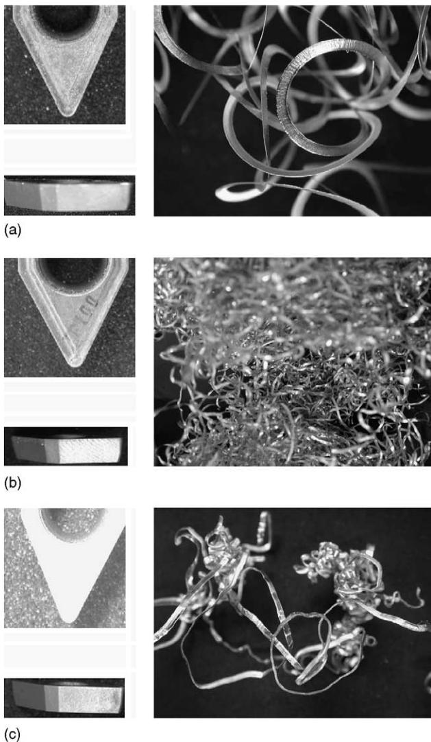
Fig. 7. Macrograph of the used tools and obtained chips during the processes made under the next conditions:  $v = 85$  m/min and: (a)  $a = 0.05$  mm/rev; (b)  $a = 0.10$  mm/rev and (c)  $a = 0.30$  mm/rev.
