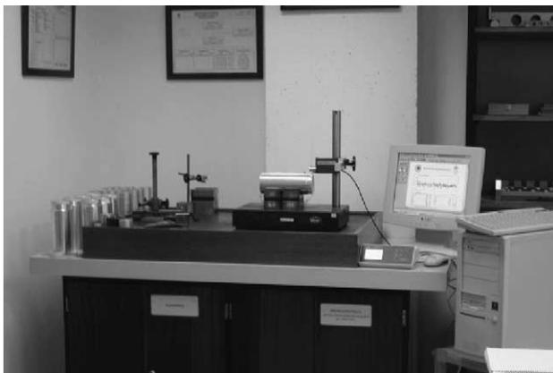
Fig. 2. Roughness measurement equipment layout.
