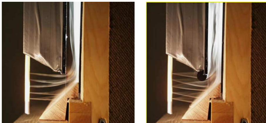
Fig. 4. Visualisation of flow at inlet with no profile (left) and when the glass edge is provided with circular profile of radius 6 mm (right).
