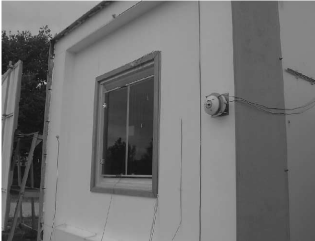
Fig. 5. The SOLVENT window installed in the PASLINK test cell at Cottbus, summer configuration.
