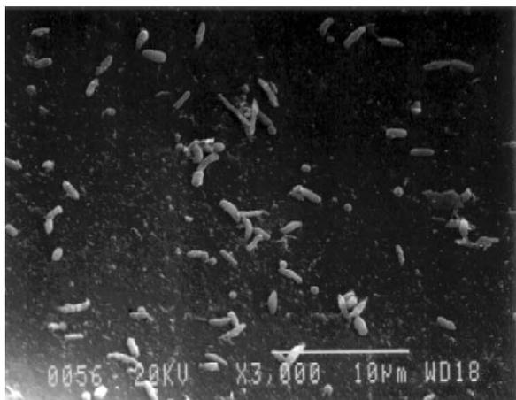
Fig. 11. Photomicrograph (SEM  $\times 3000$ ) of the surface of POLYURETHANE FOAM with immobilized acetic acid bacteria.
