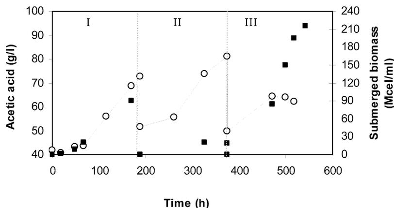
Fig. 13. Experimental data of acetic acid concentration ( $\circ$ ) and submerged biomass ( $\blacksquare$ ) vs. time during the fermentation cycles with immobilized acetic acid bacteria on WOOD CHIPS.
