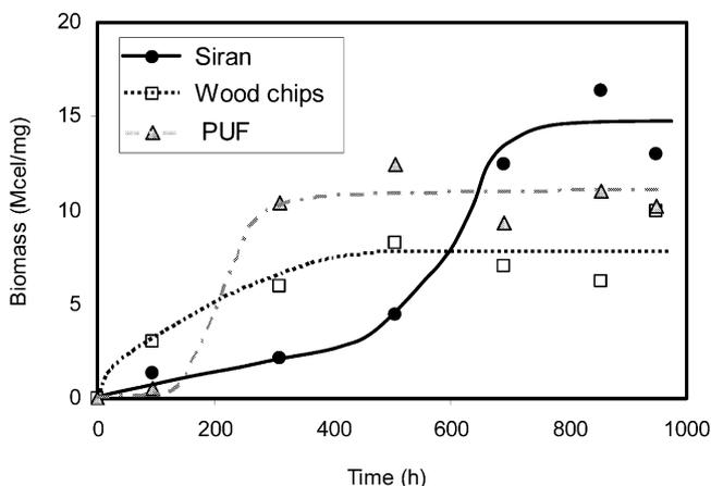
Fig. 8. Experimental data of immobilized biomass in Mcel/mg (millions of cells per milligram of carrier) vs. process time (h), for the three assayed carriers.
