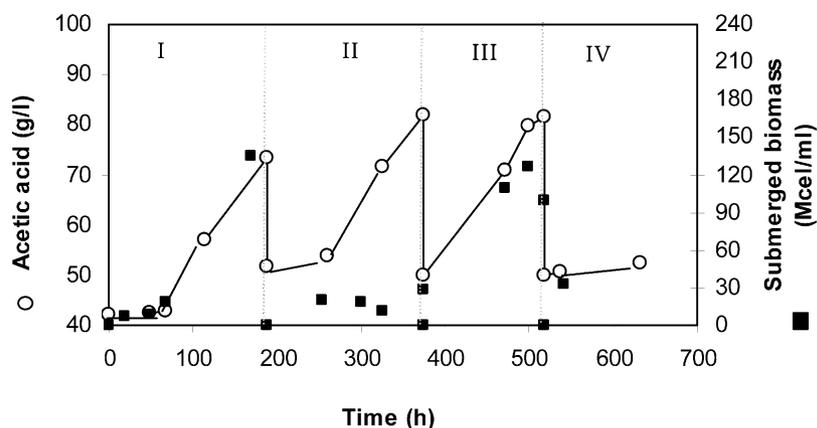
Fig. 12. Experimental data of acetic acid concentration ( $\circ$ ) and submerged biomass ( $\blacksquare$ ) vs. time during the fermentation cycles with immobilized acetic acid bacteria on SIRAN.
