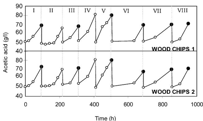
Fig. 6. Experimental data of acetic acid concentration vs. time during the immobilization cycles (I–VIII) in the laboratory reactors (WOOD CHIPS). The black dots represent the sampling points for desorption and re-count.
