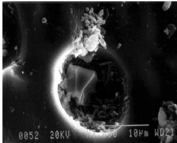
Fig. 9. Photomicrograph (SEM  $\times 3000$ ) of a micropore structure in a unit of SIRAN with immobilized acetic acid bacteria.
