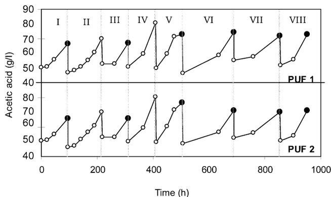
Fig. 7. Experimental data of acetic acid concentration vs. time during the immobilization cycles (I–VIII) in the laboratory reactors (POLYURETHANE FOAM). The black dots represent the sampling points for desorption and re-count.
