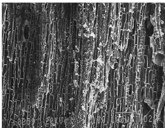
Fig. 3. Longitudinal ( $\times 130$ ) and transversal ( $\times 200$ ) cuts in WOOD CHIPS units assayed.
