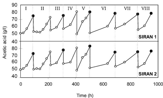
Fig. 5. Experimental data of acetic acid concentration vs. time during the immobilization cycles (I–VIII) in the laboratory reactors (SIRAN). The black dots represent the sampling points for desorption and re-count.
