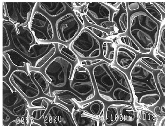
Fig. 4. POLYURETHANE FOAM internal structure ( $\times 50$ ).
