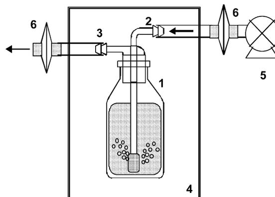
1. Glass reactor with 500 mL total capacity and 450 mL working volume
