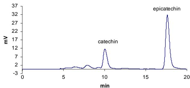
Fig. 2. Chromatogram of an extract obtained by PLE of non-fermented tea leaves. Fluorescence detection conditions: excitation, 290 nm; emission, 320 nm.
