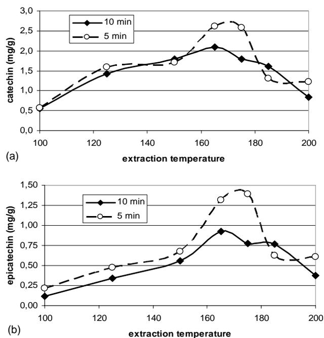
Fig. 3. Recoveries for catechin (a) and epicatechin (b) from grape seeds during the pressurized liquid extraction at different temperatures using two different extraction times: 5 and 10 min.
