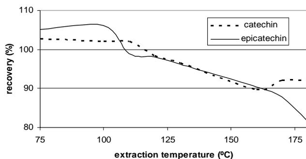
Fig. 4. Recoveries for catechin (a) and epicatechin (b) standards during the pressurized liquid extraction at different temperatures.
