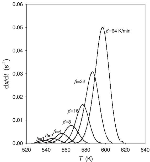
Fig. 2. Crystallization rate versus temperature for the as-quenched glass at different heating rates.
