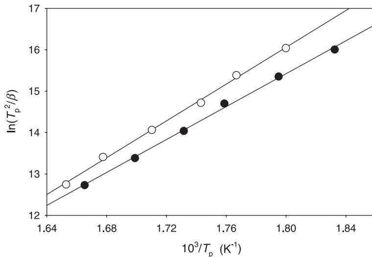
Fig. 3. Experimental plots of  $\ln(T_p^2/\beta)$  versus  $10^3/T_p$  and straight regression lines of the  $\text{Sb}_{0.04}\text{As}_{0.48}\text{Se}_{0.48}$  alloy ( $\beta$  in  $\text{K s}^{-1}$ ): (●) as-quenched glass; (○) reheated glass.
