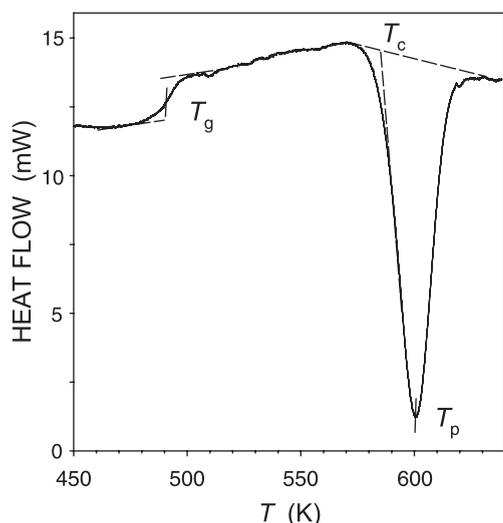
Fig. 1. DSC trace of the  $\text{Sb}_{0.04}\text{As}_{0.48}\text{Se}_{0.48}$  glassy alloy at a heating rate of  $64 \text{ K min}^{-1}$ .
