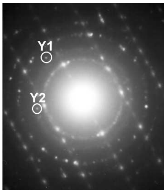
FIGURE 11 HREM images of samples implanted with N + + B + + C + annealed at 1200 °C for 3 h. Spots Y 1 and Y 2 correspond to crystalline inclusions in layer 1
