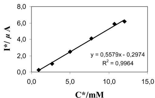
**Fig. 4** Calibration plot of  $I^*$  ( $\mu\text{A}$ ) against cysteine concentration ( $C^*$ ).  $I^*$  is the chronoamperometric current measured a fixed, short time after polarization, for each addition of substrate, with the background contribution subtracted;  $C^*$  is the concentration corrected for dilution
