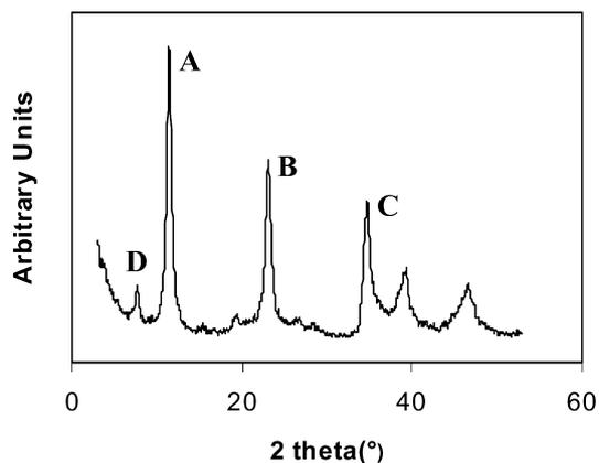
Fig. 5 XRD pattern of the [Mg/Al-CoTSPc] HT
