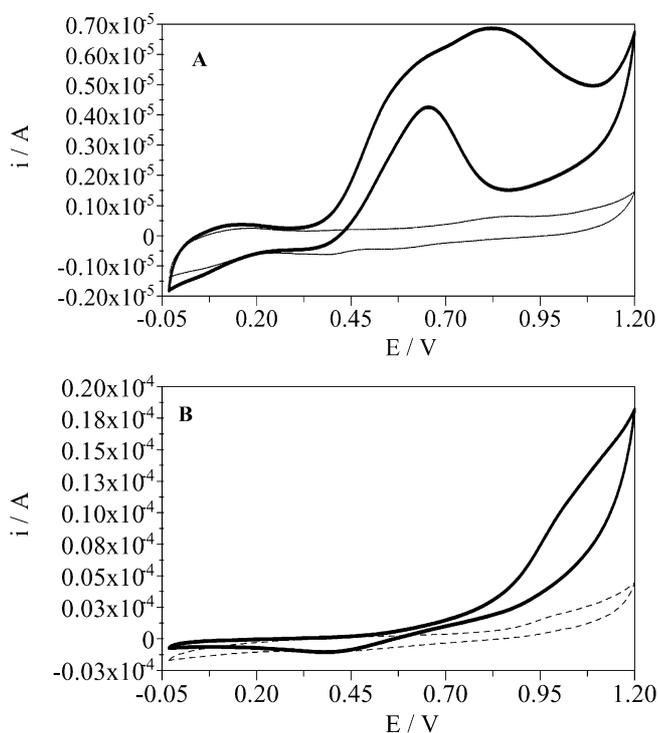
**Fig. 3** Cyclic voltammograms obtained from (A) SCC–CoPc10% and (B) SCC electrodes before (dotted line) and after (full line) addition of cysteine ( $1.10 \times 10^{-2} \text{ mol L}^{-1}$ ). Supporting electrolyte  $0.05 \text{ mol L}^{-1} \text{ H}_2\text{SO}_4$ ; potential scan rate  $0.05 \text{ V s}^{-1}$
