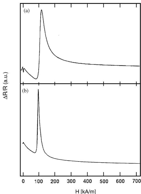
Fig. 4. Microwave absorption at 9.67 GHz, showing the FMR and FMAR peaks, for (a)  $x = 6$  and (b)  $x = 2$  amorphous microwires.
