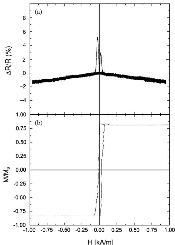
Fig. 3. (a) Microwave losses curve at 9.67 GHz and (b) hysteresis loop for the  $x = 10$  microwire.
