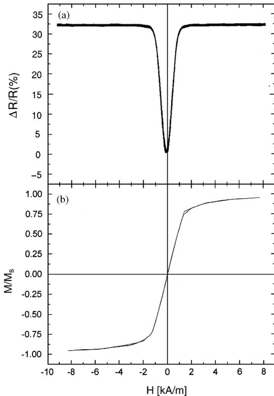
Fig. 1. (a) Microwave magnetoimpedance curve at 9.67 GHz and (b) hysteresis loop for the  $(\text{Co}_{98}\text{Fe}_2)_{75}\text{Si}_{15}\text{B}_{10}$  microwire.
