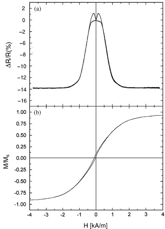
Fig. 2. (a) Microwave magnetoimpedance at 9.67 GHz and (b) hysteresis loop for the  $x = 6$  microwire.
