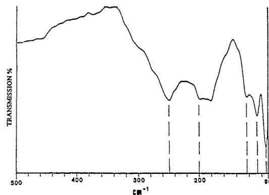
Fig. 1. Infrared transmission spectrum of  $\text{Ge}_{0.20}\text{Sb}_{0.05}\text{Se}_{0.75}$  glass.
