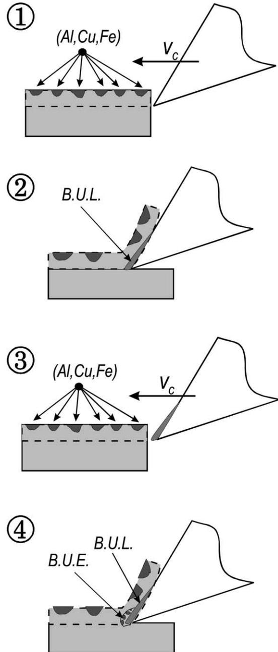
Fig. 10. Scheme of the BUL (a) and (b) and BUE (c) and (d) formation.
