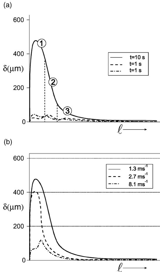
Fig. 5. Profiles recorded on the metal adhered onto the insert surfaces turned: (a) at 80 m/min during the indicated periods; (b) during 10 s at the indicated cutting speeds.
