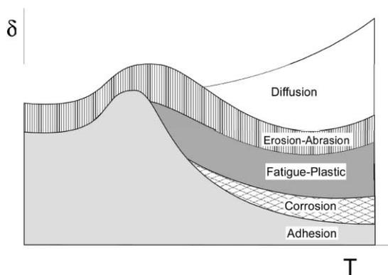
Fig. 1. Wear mechanisms as a function of temperature.
