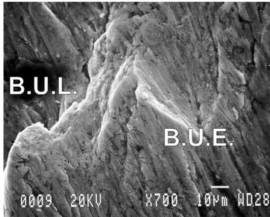
Fig. 7. SEM image acquired on the frontier between BUL and BUE.
