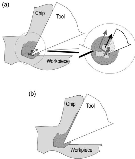
Fig. 2. (a) BUE formation mechanism and wear by adhesion. (b) Tool with BUE and BUL.
