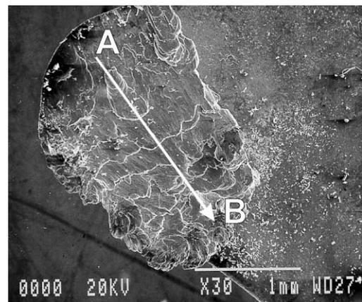
Fig. 4. SEM image acquired on a tool insert after 10 s turning test at 80 m/min.
