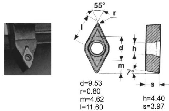
Fig. 3. Tool insert employed in the experimental study.
