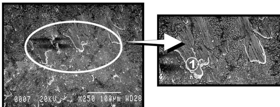
Fig. 6. Detail of BUL formed on the insert surface after a second turning test.
