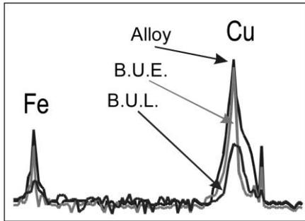
Fig. 9. Detail of the Fe and Cu peaks of the EDS spectra included in Fig. 8.
