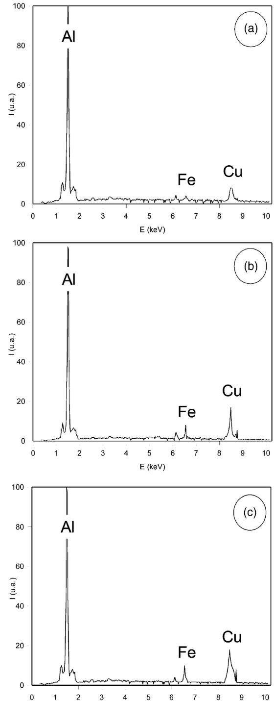
Fig. 8. EDS spectra recorded on: (a) BUL, (b) BUE and (c) alloy AA2024.
