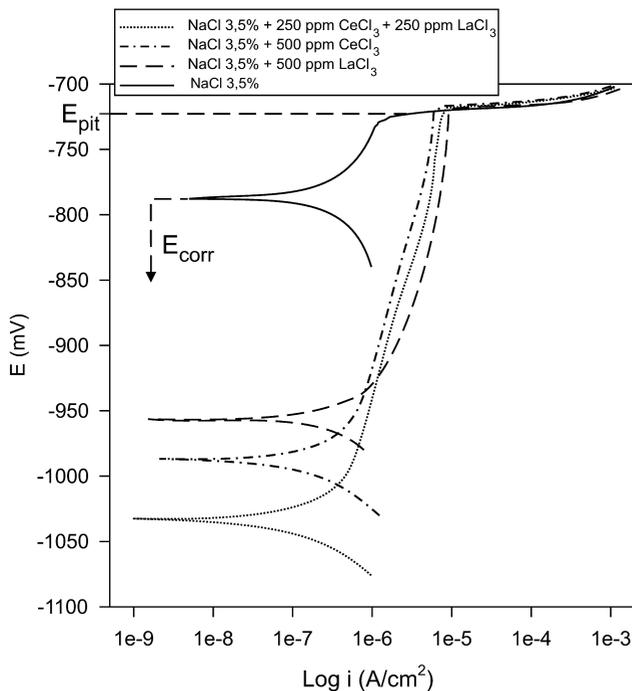
Fig. 1. Linear polarisation curves for AA5083 in bare NaCl solution and with different additions of  $\text{LnCl}_3$ .
