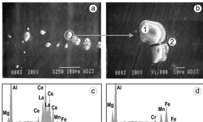
Fig. 4. (a) SEM image recorded on a sample of the AA5083 alloy after 2 h of immersion in 250 ppm CeCl<sub>3</sub> + 250 ppm LaCl<sub>3</sub>; (b) high magnification view of one of the nodules observed in (a); (c) EDS spectrum recorded in (1); (d) EDS spectrum recorded in (2).
