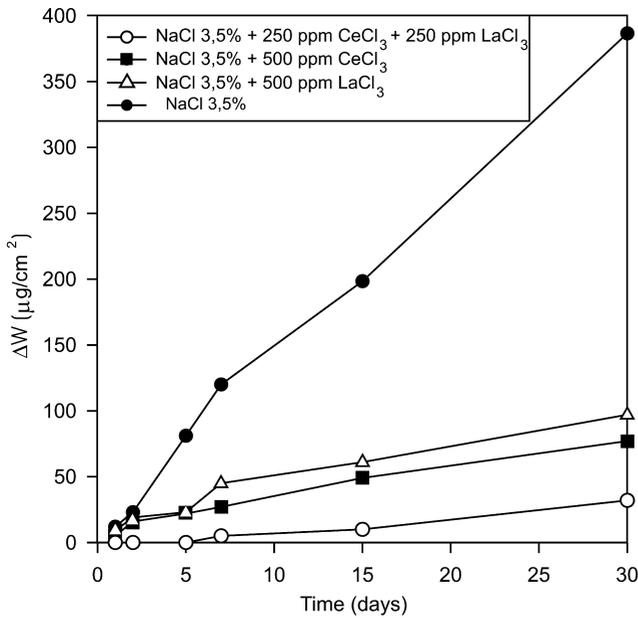
Fig. 3. Weight loss–time curves of full immersed samples of AA5083 in 3.5% NaCl aerated solutions. The highest decrease in weight loss is observed for the CeCl<sub>3</sub>/LaCl<sub>3</sub> mixture.
