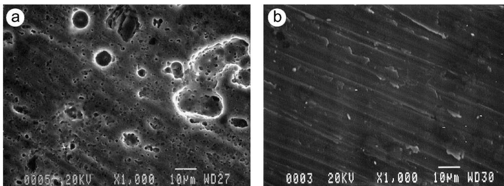
Fig. 5. SEM micrographs, of cleaned AA5083 samples after 30-day full immersion tests in (a) bare NaCl 3.5% solution and (b) doped with 250 ppm  $\text{CeCl}_3$  + 250 ppm  $\text{LaCl}_3$ .
