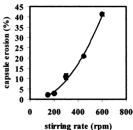
Fig. 2. Relationship between stirring rate and percentage of capsule disintegration.
