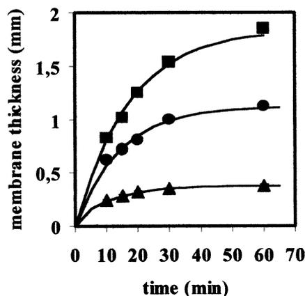
Fig. 1. Effects of gelation time,  $\text{CaCl}_2$  and sodium alginate concentration on membrane thickness of capsules. Symbols: (●) sodium alginate 1.0% w/v and  $\text{CaCl}_2$  5.5% w/v; (■) sodium alginate 0.5% w/v and  $\text{CaCl}_2$  5.5% w/v; (▲) sodium alginate 0.5% w/v and  $\text{CaCl}_2$  1.3% w/v.
