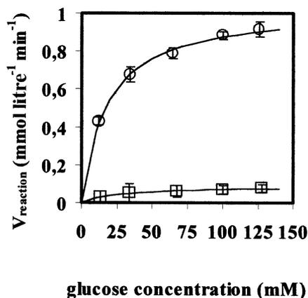
Fig. 3. Reaction rates of free (●) and encapsulated GOD (■) at different glucose concentrations. pH 5.1; temperature 35°C; 0.019 g free enzyme or 0.146 g GOD-immobilized calcium alginate gel capsules.
