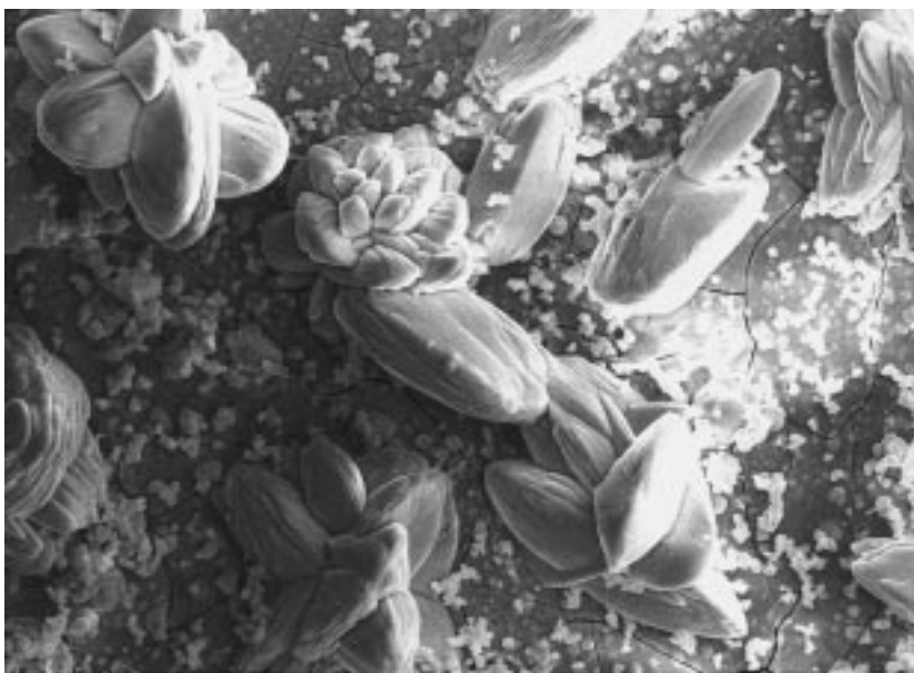
Fig. 11. SEM image of large cerium precipitates created in the galvanised steel surface after 30 days in 3.56% NaCl solution with 250 ppm \text{CeCl}_3 ( \times 500 ).
