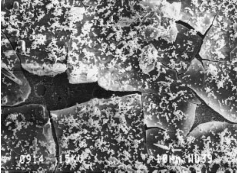
Fig. 9. Surface appearance of galvanised steel after 30 days of immersion in 3.56% NaCl solution with 500 ppm CeCl 3 .
