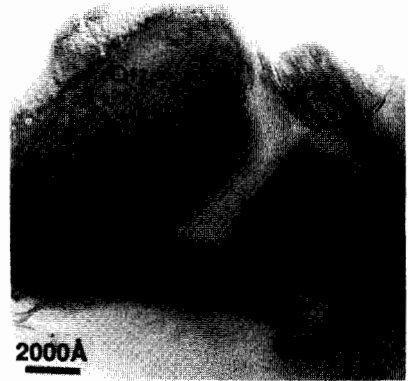
Fig. 3. Low-magnification (45000 \times ) TEM image showing the typical texture of sample 265. Detrital quartz (Qtz) and kaolinite (Kln) grains are embedded in a fine-grained matrix of phyllosilicates.
