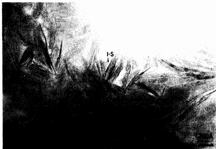
Fig. 7. Lattice-fringe image of small, curled I-S flakes neofomed in pore space; 10 and 20-Å fringes are present (sample 256).
