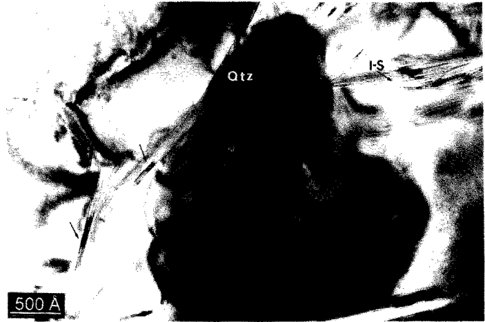
Fig. 10. TEM image of 477-m deep sample showing both detrital and authigenic phases. Neoformed small I-S packets occur in the matrix (thin arrows), near a corroded detrital quartz grain (Qtz).
