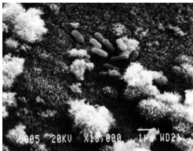
Fig. 4 Scanning electron micrograph of biomass support particles removed during immobilisation process
