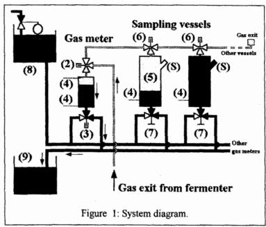
gases, while the lower controls the entry and exit of the displacement liquid (0.48cm diam, model K92922). The three terminals of the level detectors (upper level, lower level and common) are conductive points and their relative position in the receptacle marks the volume measured in each cycle of the system. The sampling vessels have one level sensor and a septum (S).
