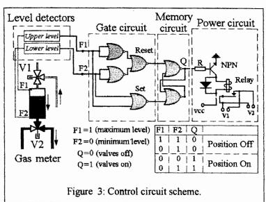
The gate circuit and the memory circuit use NOR logic gates and the table of truth is shown in figure 3. The power circuit has only one outlet since the two selenoid valves operate in unison. The control system for the sampling simply comprises commercial timing devices (one for each receptacle), to which are connected the corresponding selenoid valves to open and close at the pre-set time.
