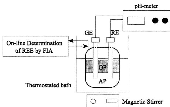
Fig. 1. Schematic representation of experimental manifold. OP: organic phase; AP: aqueous phase; GE: glass electrode; RE: reference electrode.
