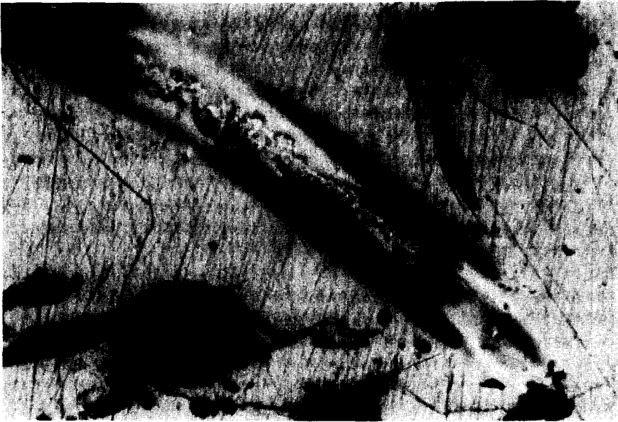
Fig. 6. Photomicrograph ( \times 35 ) of a switch-on path enclosing a partially developed filament.
