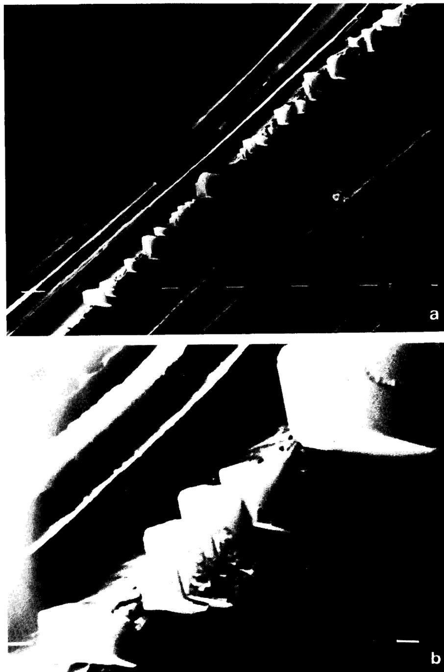
Fig. 4. Calcite rhombohedral crystals forming the outer part of an IMCA with a whole morphology as in fig. 2a: (a) scale bar 5  $\mu\text{m}$ ; (b) enlarged view of (a); scale bar 0.5  $\mu\text{m}$ .
