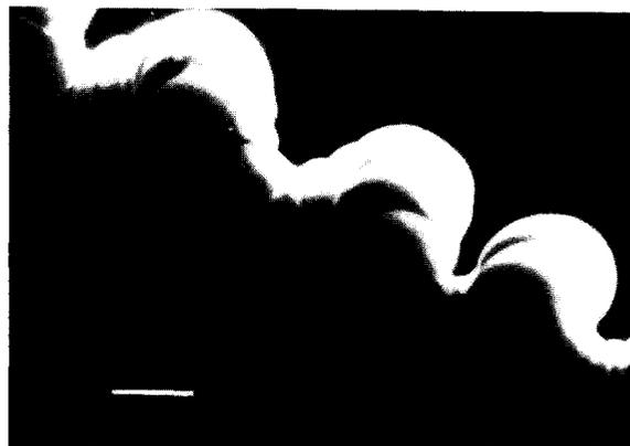
Fig. 7. Twisted ribbon obtained when increasing the carbonate concentration. IMCA of  $\text{BaCO}_3$ . Scale bar 0.2 mm.
