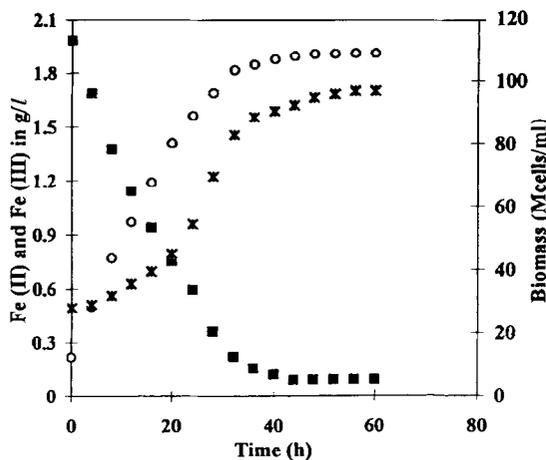
FIG. 5. Experimental data of ferrous iron, ferric iron and biomass versus time at 35°C. Symbols: ■, Fe (II); ○, Fe (III); ●, biomass.
