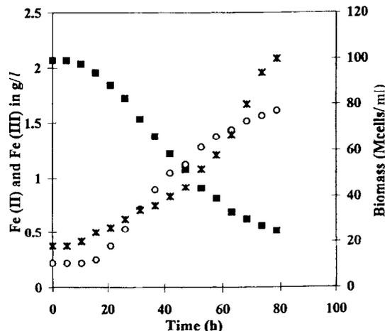
FIG. 2. Experimental data of ferrous iron, ferric iron and biomass versus time at 20°C. Symbols: ■, Fe (II); ○, Fe (III); ●, biomass.
