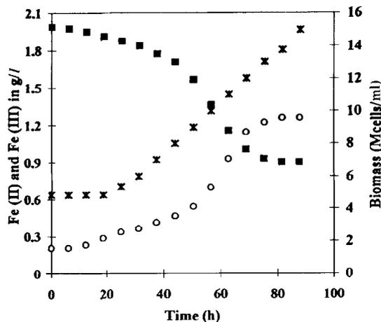
FIG. 1. Experimental data of ferrous iron, ferric iron and biomass versus time at 15°C. Symbols: ■, Fe (II); ○, Fe (III); ●, biomass.
