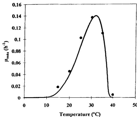
FIG. 7. Theoretical predictions and experimental data of maximum specific growth rate ( $\text{h}^{-1}$ ) for *T. ferrooxidans* versus temperature. Symbols: ●, experimental; —, theoretical.
