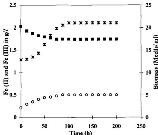
FIG. 6. Experimental data of ferrous iron, ferric iron and biomass versus time at 40°C. Symbols: ■, Fe (II); ○, Fe (III); ●, biomass.
