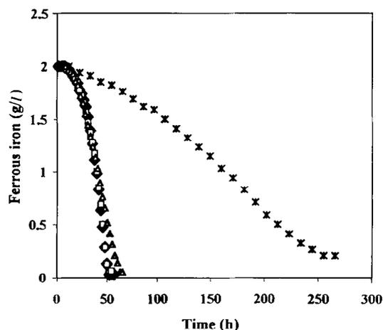
FIG. 8. Experimental data of ferrous iron versus time at different pH values. Symbols:  $\blacklozenge$ , pH 2.5;  $\square$ , pH 2.0;  $\triangle$ , pH 1.5;  $\bullet$ , pH 1.25.
