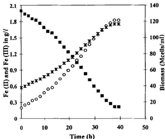
FIG. 4. Experimental data of ferrous iron, ferric iron and biomass versus time at 30°C. Symbols: ■, Fe (II); ○, Fe (III); ●, biomass.
