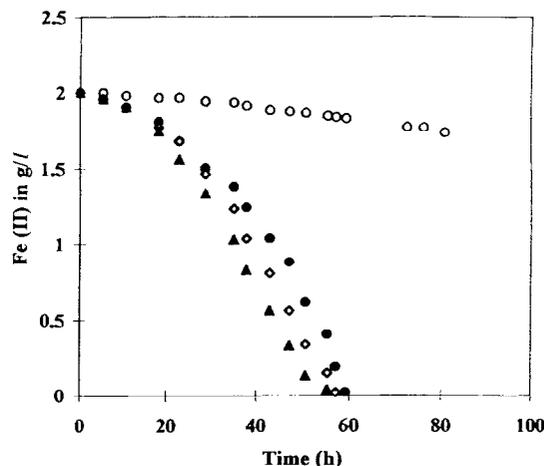
FIG. 10. Experimental data of ferrous iron versus time at different agitation rates. Symbols:  $\circ$ , 0 rpm;  $\bullet$ , 100 rpm;  $\diamond$ , 200 rpm;  $\blacktriangle$ , 250 rpm.
