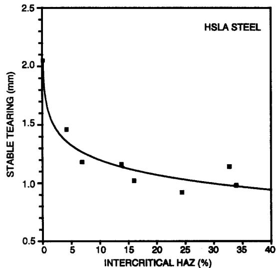
Fig. 4. Subcritical crack growth versus percentage of intercritical HAZ.
