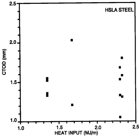
Fig. 2. Crack tip opening displacement versus heat input of weldment.
