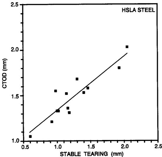
Fig. 3. Linear regression of CTOD versus subcritical crack growth.
