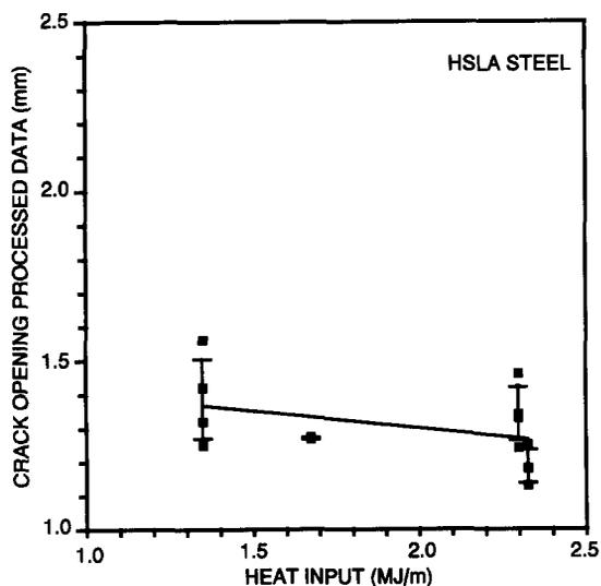
Fig. 7. Modified crack tip opening displacement versus heat input of weldment.
