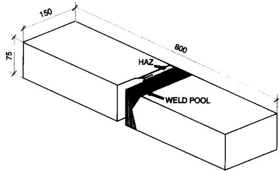
Fig. 1. Schematic of K-shaped butt weld joint.
