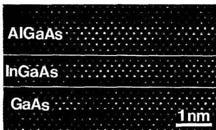
Fig. 3. [110] HREM image of the InGaAs channel layer.
