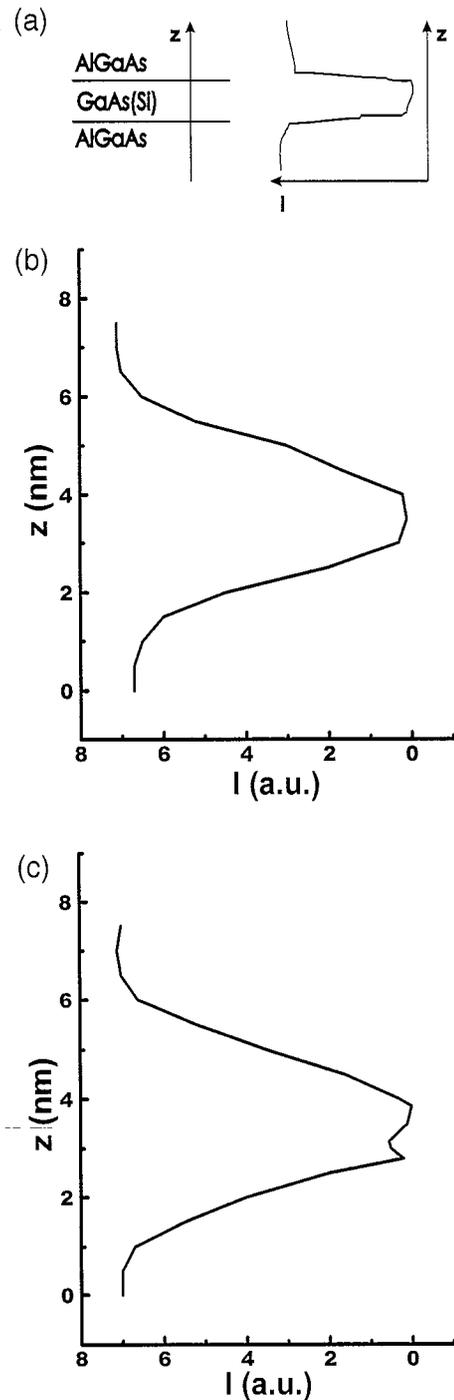
Fig. 2. Profile analysis of the Si  $\delta$ -doped GaAs layer. (a) Profile acquisition; (b) most usual obtained profile; (c) exceptionally obtained profile.
