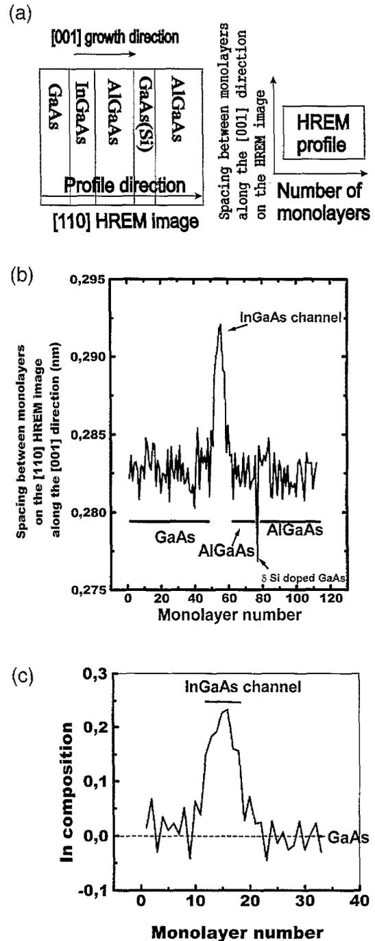
Fig. 4. Analysis of [110] HREM images. (a) Acquisition procedure of profiles for strain measurements. (b) Example of spacing profile containing a strong signal in the GaAs(Si) layer. (c) Composition profile obtained from the spacing profile of (b) in the InGaAs channel.
