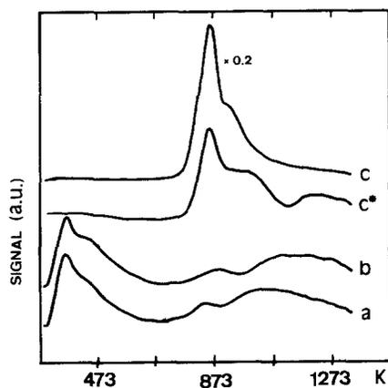
Fig. 2. Temperature-programmed desorption of hydrogen after reduction of samples a, b and c at 773 K, cooling under flow of argon, and treatment with a flow of hydrogen ( $1 \text{ cm}^3 \text{ s}^{-1}$ ) at ambient temperature. c\* corresponds to the signal recorded for sample c, reduced at 773 K and cooled under flow of argon without further treatment with hydrogen. Note that signal c has been divided by a factor of 5. (Heating rate:  $0.17 \text{ K s}^{-1}$ .)
