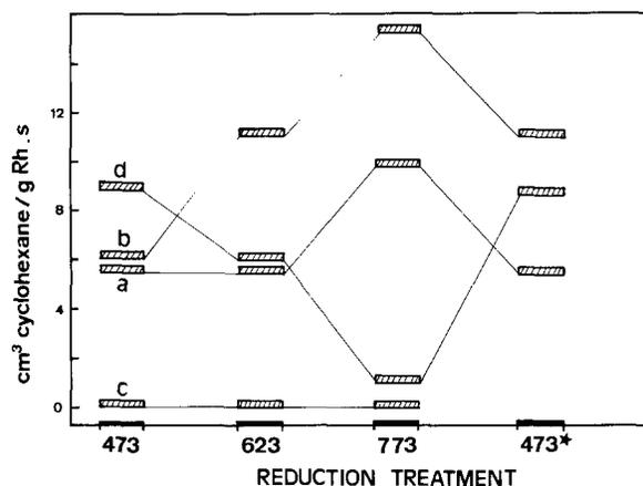
Fig. 3. Catalytic activities, corresponding to catalysts a, b, c and d, for the benzene hydrogenation reaction, after reduction at different temperatures (473, 623 and 773 K). 473\* represents the catalytic activities observed for the samples reduced at 773 K, reoxidized in air at 673 K, and further reduced in hydrogen at 473 K.
