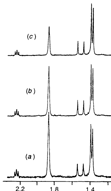
Fig. 6 Methyl region of 1 H NMR spectra taken during the decomposition of trans -[Mo(N 2 ) 2 (PPh 2 Me) 4 ] in the presence of an excess of phosphine ([I] = 2.0 \times 10^{-3} mol dm -3 and [PPh 2 Me] = 5.0 \times 10^{-3} mol dm -3 ). In spectrum (a) acquisition was started immediately after complex 1 was completely dissolved; (b) and (c) acquisition was started 30 and 60 min later, respectively
