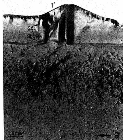
Fig. 7. Topograph of Z-4 plate of crystal QS-2 showing the different growth regions of trapezohedral subsector 1' Sb_3 GSB exhibits a strong contrast and Sb_4 GSB is also visible. 0\bar{3}31 reflection.
