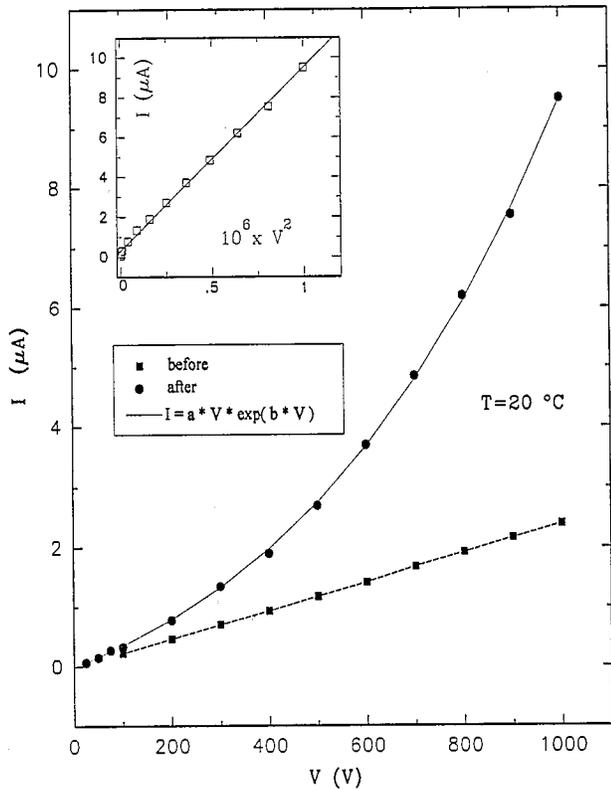
Fig. 5.  $I-V$  and  $I-V^2$  characteristics of the sample before and after the thermal switching.
