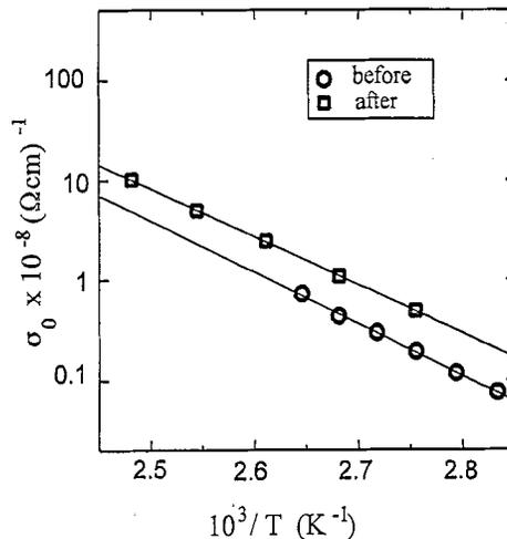
Fig. 3. Change in  $I-V$  characteristics and in the pre-exponential factor of Eq. (3), for the compound  $\text{Ge}_3\text{Se}_3\text{Te}_4$ , produced by forced ageing of the sample under 120 °C.
