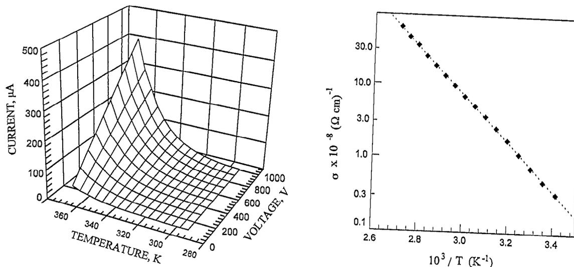
Fig. 1.  $I$ – $V$ – $T$  characteristics and variation of conductivity with temperature in the initial state of glassy alloy  $\text{Ge}_3\text{Se}_3\text{Te}_4$  (sandwich electrode configuration).
