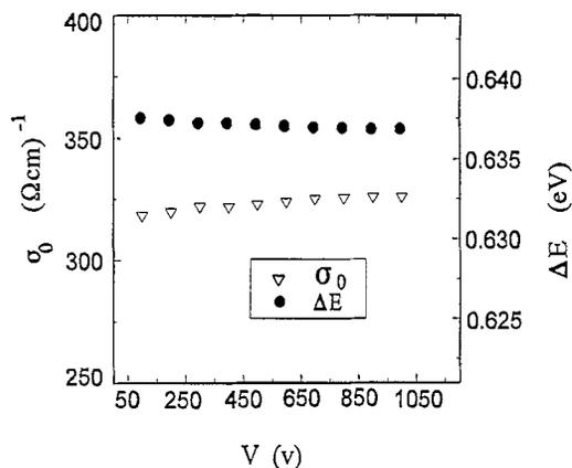
Fig. 2. Parameters  $\sigma_0$  and  $\Delta E$  calculated for different applied voltages, according to Eq. (3).
