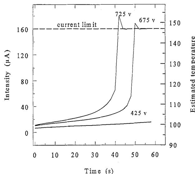
Fig. 4. Switching processes carried out with limited current. Temperature on the right axis was estimated from Eq. (2).
