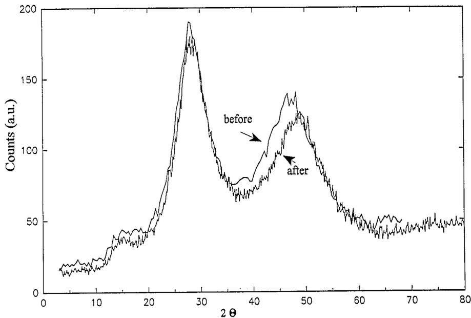
Fig. 6. X-ray diffractograms for the sample under study before and after the electrothermal annealing.
