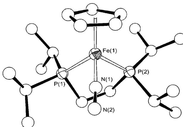
Figure 9. Molecular structure of the cationic dinitrogen complex  $[\text{CpFe}(\text{N}_2)(\text{dippe})]^+$
