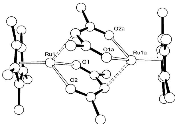
Figure 5. Molecular structure of the dimer  $[\{\text{Cp}^*\text{Ru}(\text{acac})\}_2]$
