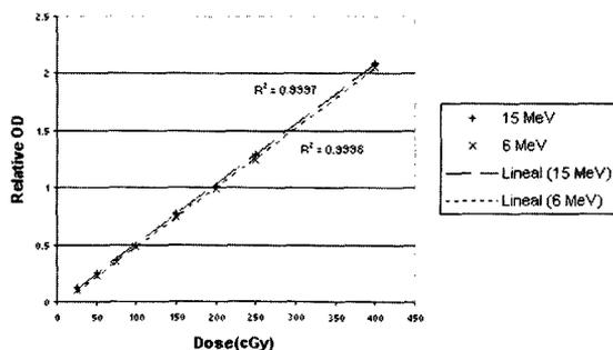
Kodak EDR2 have been irradiated at measurement depths of IAEA TRS-398 protocol in a PTW RW3 laminar solid water phantom with nominal electron energies of 6 and 15 MeV and a circular applicator of 5 cm diameter. Doses of 25, 50, 75, 100, 150, 200, 250 and 400 cGy were delivered to develop the characteristic curve for the EDR2 film for each beam energy. Calibration procedure shows a OD to dose linear response using both digitiser and a X-RITE desk
