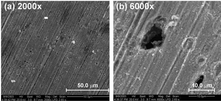
Fig. 3. SEM micrograph of typical pits after removing the corrosion products in API-5XL52 alloy at (a) 2000 $\times$  and (b) 6000 $\times$ ; 45 days of immersion in medium with bacteria and thiosulfate.
