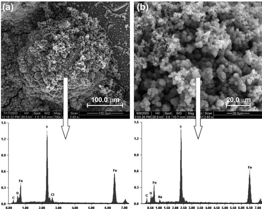
Fig. 2. SEM image of deposits on the surface of API-5XL52 alloy and EDS spectra of these deposits, at: (a) 7 days and (b) 45 days of immersion in medium with bacteria and thiosulfate.
