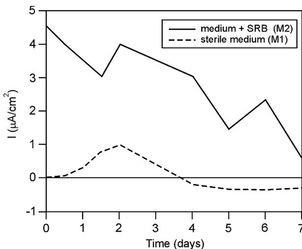
Fig. 7. Averaged density current from ENM of API-5XL52 alloy, in function of the exposure time in presence (M2) and absence (M1) of bacteria.
