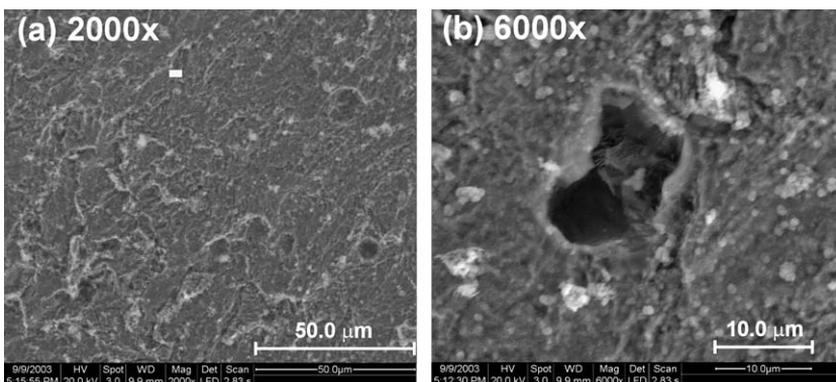
Fig. 4. Typical pits seen after removal of corrosion products in St-35.8 alloy at (a) 2000 $\times$  and (b) 6000 $\times$ ; 45 days of immersion in medium with bacteria and thiosulfate.
