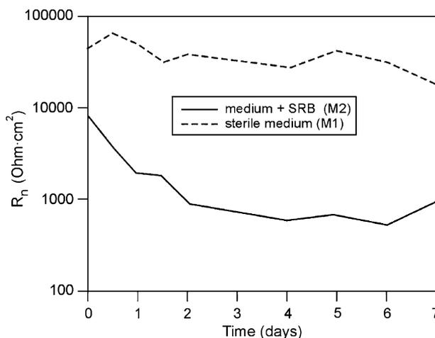
Fig. 8. Noise resistance values of API-5XL52 alloy, in function of the exposure time in presence (M2) and absence (M1) of bacteria.
