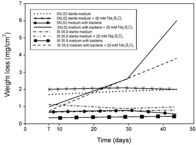
Fig. 1. Weight loss-time curves of full immersion of St-35.8 and API-5XL52.
