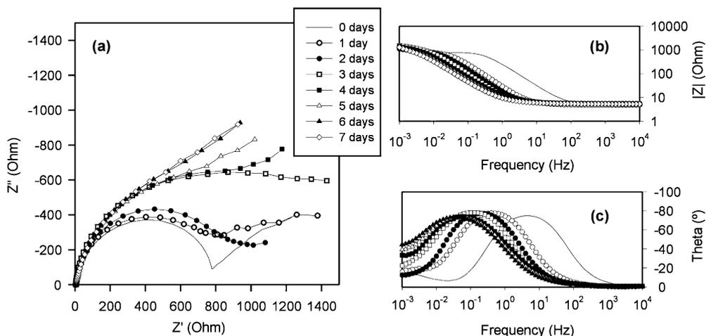
Fig. 9. Impedance diagrams of API-5XL52 samples immersed in M1 media for 7 days. (a) Nyquist diagram, (b) Bode modulus diagram and (c) Bode phase angle diagram.
