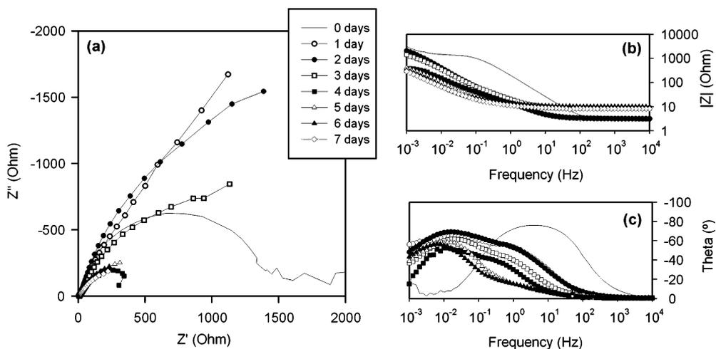
Fig. 10. Impedance diagrams of API-5XL52 samples immersed in M2 media (sterile media + SRB + thiosulfate) for 7 days. (a) Nyquist diagram, (b) Bode modulus diagram and (c) Bode phase angle diagram.
