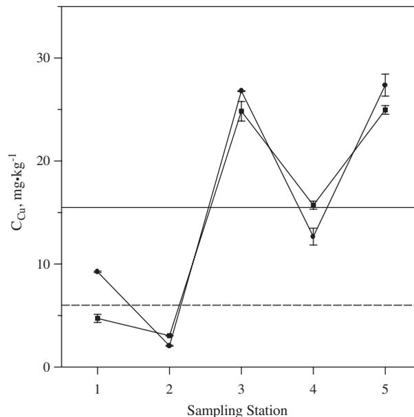
Fig. 3. Concentration of Cu in the sediments of San Pedro River. Error bars indicate standard deviations of two replicates. ●: 1997; ■: 1998; dashed line indicates Cu concentration in sandstone. Solid line indicates Cu concentration in the culture pond.
