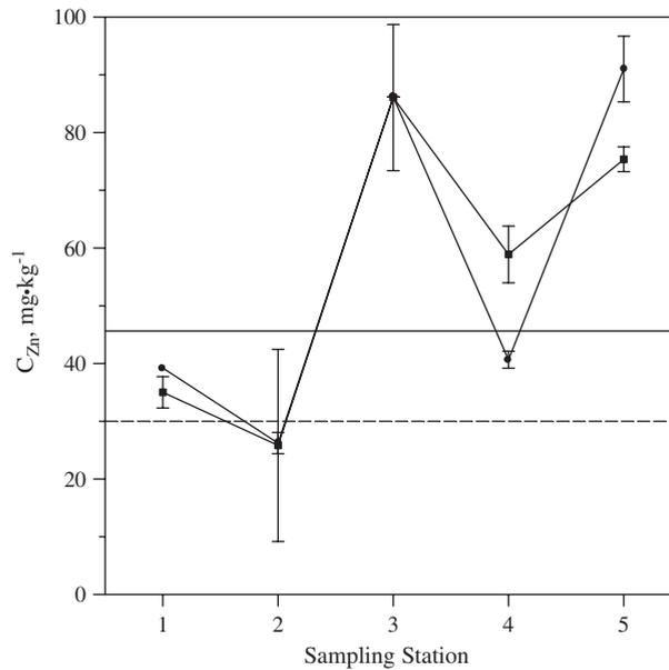
Fig. 2. Concentration of Zn in the sediments of San Pedro River. Error bars indicate standard deviations of two replicates. ●: 1997; ■: 1998; dashed line indicates Zn concentration in sandstone. Solid line indicates Zn concentration in the culture pond.
