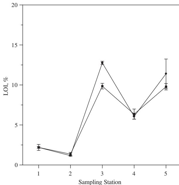
Fig. 5. Contents of organic matter (as Loss on Ignition) in the sediments of San Pedro River. Error bars indicate standard deviations of two replicates. ●: 1997; ■: 1998.
