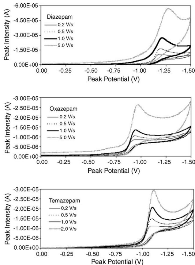
Fig. 3. Cyclic voltammograms at different values of scan rate for the three benzodiazepines.
