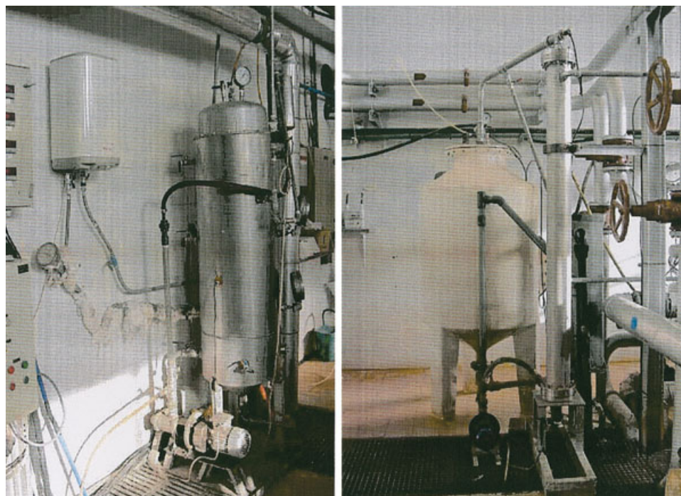
Figure 1. 175 L Pilot-plant digester (CSTR1), and 850 L Pilot-plant digester (CSTR2).
