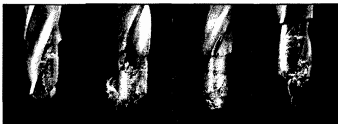
Fig. 5. Material accumulated in WC-10Co tools after dry drilling AA2024 alloy.
