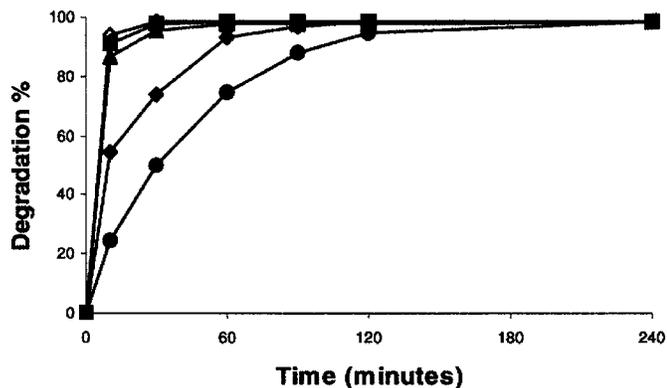
**Fig. 3.** Primary degradation percentage of PCBs using different molar ratios with iron ions:  $R=(\blacklozenge)$  1000,  $(\blacksquare)$  100,  $(\blacktriangle)$  10,  $(\bullet)$  0 (without  $H_2O_2$ ), and  $(\diamond)$   $R=100$  without Fe
