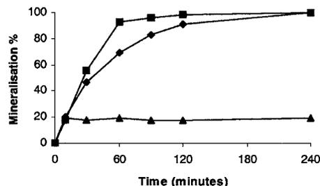
**Fig. 4.** Mineralization percentage of LAS+PCBs using different molar ratios with or without iron ions:  $R=(\blacklozenge)$  100 with Fe ions  $(\blacksquare)$  100 without Fe, and  $(\blacktriangle)$  10 with Fe ions
