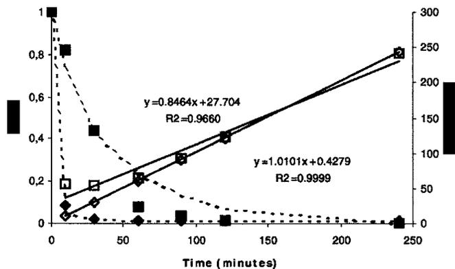
**Fig. 6.** Linear fit obtained with the Chan-Chu kinetic model. Experimental data: ( $\blacklozenge$ ,  $\blacklozenge$ ) primary degradation and ( $\blacksquare$ ,  $\square$ ) mineralization. Theoretical values: ( $\cdots$ ) and ( $—$ ).
