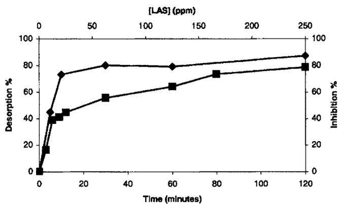
**Fig. 1.** Evolution of the PCB desorption percentage (◆) and of the luminescence inhibition (toxicity) (■)
