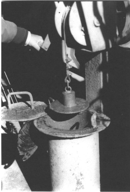
Fig. 1. Detail of sounding lead used to measure distance between deck and sand surface. Flat shape allows device to lie directly on top of sediment surface, avoiding penetration.
