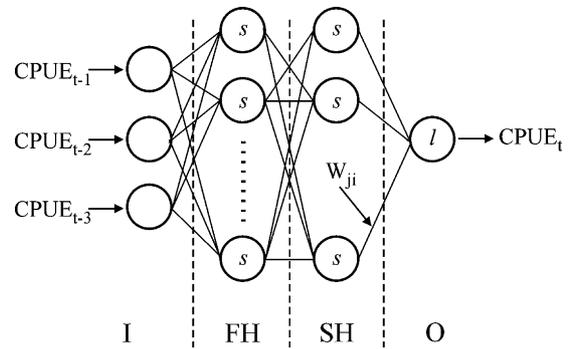
Fig. 1. Schematic representation of a four-layer feed forward artificial neural network for computing halibut CPUE.
