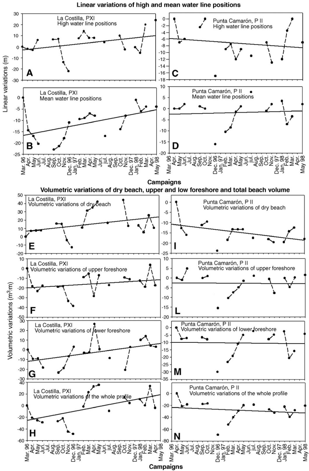
Fig. 4. Short-term evolution: examples of distances (m) surveyed from the profile benchmarks to the high and mean water levels, and volumetric variations ( $m^3/m$ ) for different parts of beach profiles and for the whole profiles.
