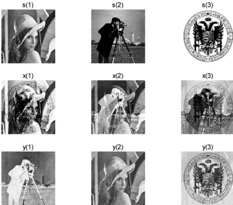
Fig. 5. Original images (s), PNL-mixtures (x) and estimations (y) applying the genetic algorithm.
