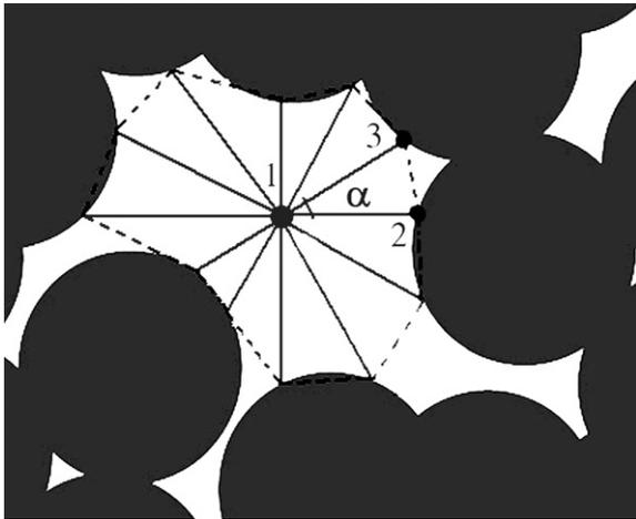
Fig. 2. Schematic illustration of the two-dimensional triangulation method applied to the pore space. Points 1, 2 and 3 correspond to the three vertices of one of the triangles.
