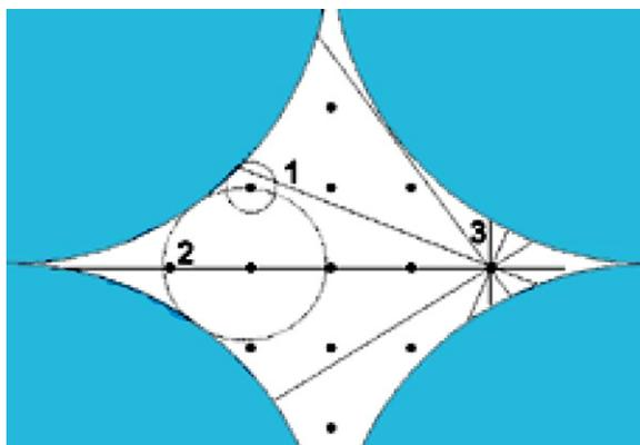
Fig. 5. 2D diagram of a grid in the pore space between 4 spheres.
