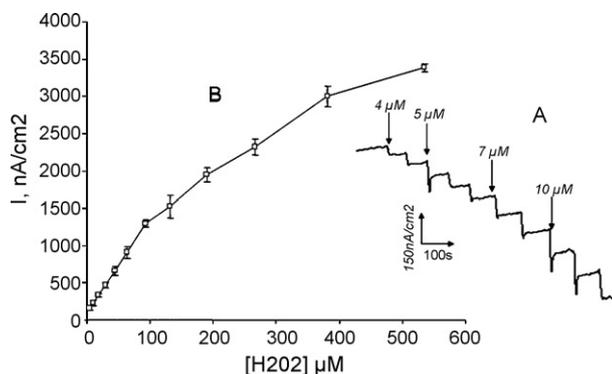
Fig. 7. Typical current-time response and calibration curves of  $\text{H}_2\text{O}_2$  recorded with the Nafion-HRP-Sonogel-Carbon biosensor at optimum conditions (pH 7 PSB and  $-250\text{ mV}$ ).
