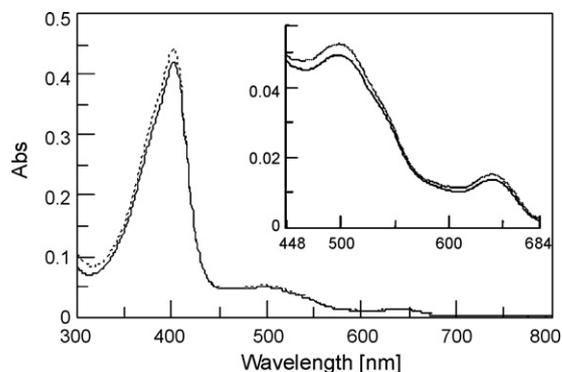
**Fig. 2.** UV-vis spectra of 0.25 mg mL<sup>-1</sup> HRP in phosphate buffer solution (solid line) and the same quantity of the enzyme crosslinked and sonicated before its solubilization (discontinuous line).
