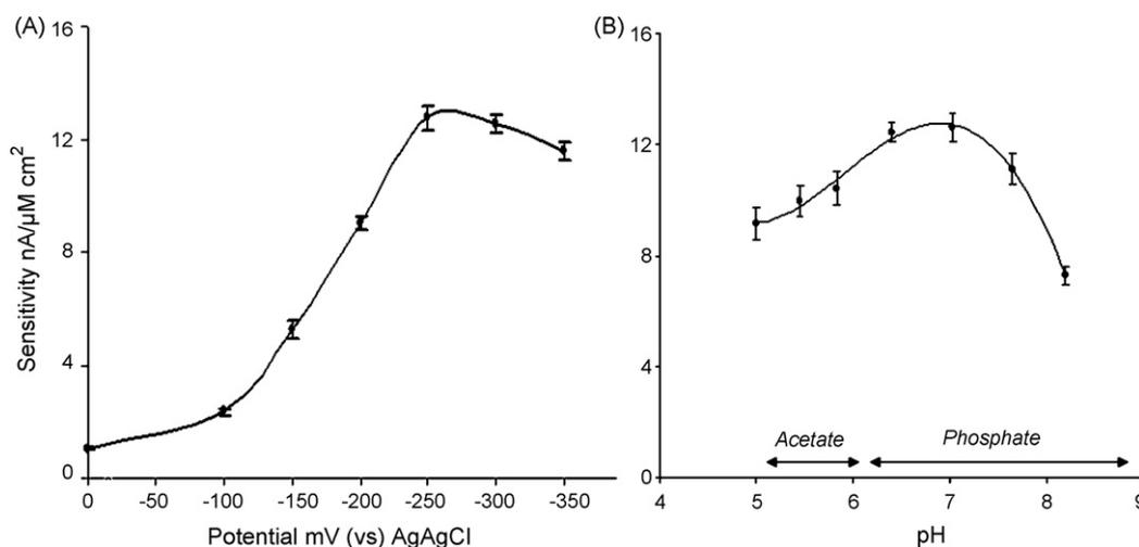
**Fig. 5.** Effect of potential (A) and pH (B) on the response of Nafion–HRP–Sonogel–Carbon biosensor. The sensitivities are deduced from steady-state current recorded at different potentials (A) and at  $-250 \text{ mV}$  (B), in  $0.05 \text{ mol L}^{-1}$  PBS.
