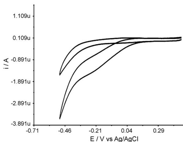
**Fig. 4.** CV of the HRP–Nafion–Sonogel–Carbon biosensor in the absence and presence of 0.5 mM  $\text{H}_2\text{O}_2$ , scan rate  $50 \text{ mV s}^{-1}$ ; other parameters are the same as in Fig. 3.
