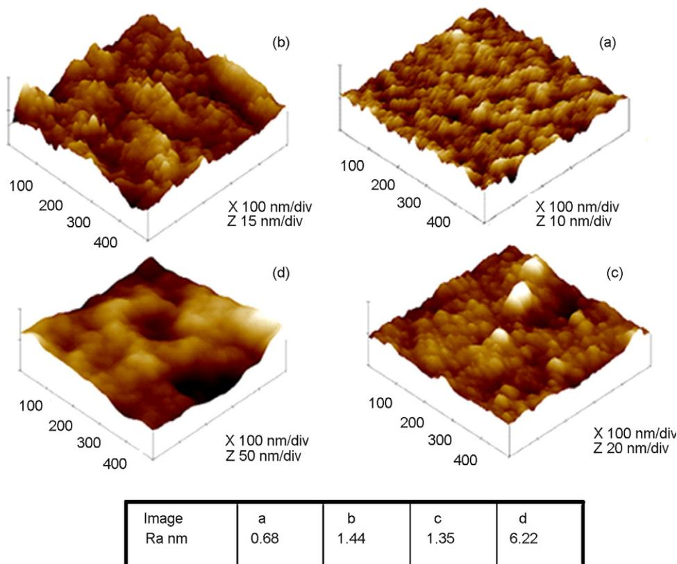
**Fig. 1.** AFM images of (a) Sonogel material, (b) Sonogel–Carbon composite, (c) Sonogel–Carbon coated by 0.5% Nafion, and (d) HRP–Nafion–Sonogel–Carbon biosensor. The table shows the corresponding roughness values.
