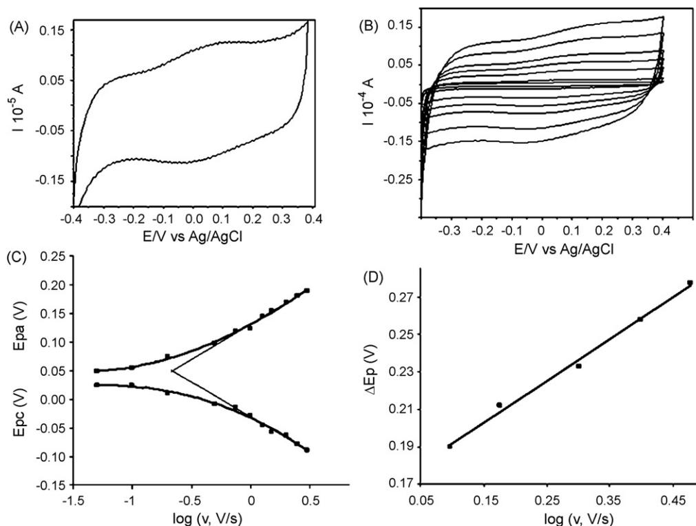
**Fig. 3.** (A) CV of native HRP–Nafion–Sonogel–Carbon biosensor at 0.2 V/s in PSB (0.05 mol L<sup>-1</sup> in both KCl and pH 7 phosphate buffer); (B) effect of scan rate from inner to outer, at 0.1, 0.2, 0.5, 0.75, 1, 1.5, and 2 V/s; (C) plots of anodic and cathodic peaks potential vs. logarithm of the scan rate; (D) plot of  $\Delta E_p$  vs.  $\log(v)$ .
