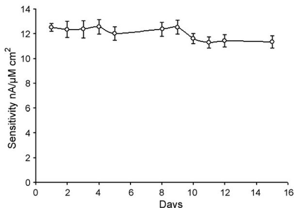
Fig. 6. Life-time profile of Nafion-HRP-Sonogel-Carbon peroxide biosensor.
