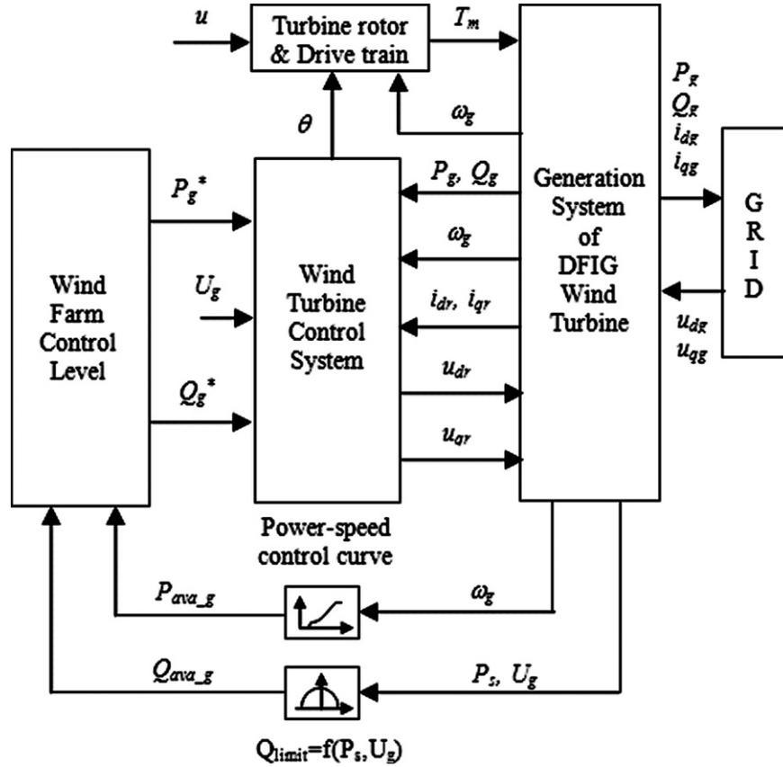
Fig. 2. Model and control system of a DFIG wind turbine.
