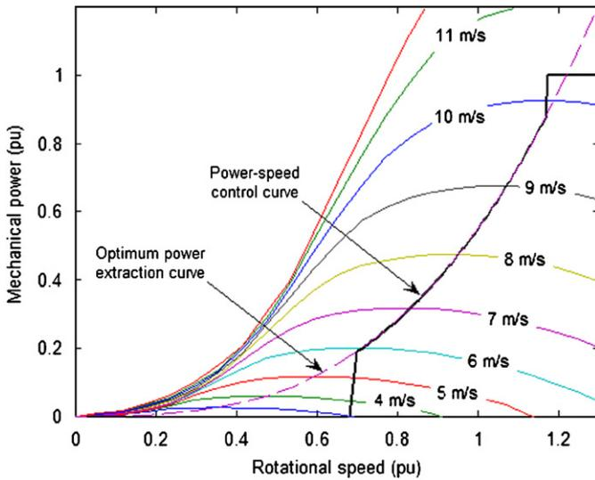
Fig. 3. Aerodynamic mechanical power, optimum power extraction curve and power-speed control curve.
