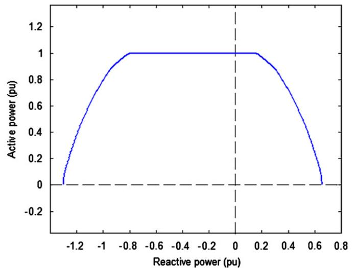
Fig. 5. Operating region of a DFIG wind turbine connected to an infinite bus.
