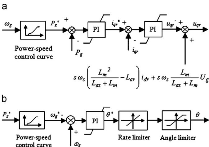
Fig. 8. Control system 2 for DFIG wind turbine: (a)  $u_{qr}$  controller (active power controller) and (b) pitch angle controller (speed controller).
