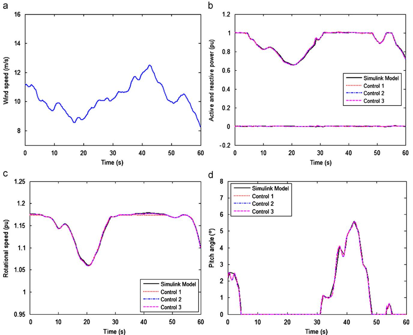
**Fig. 10.** Validation of the model and the control systems used in this work by comparison with the DFIG model wind turbine included in the SimPowerSystems library of MATLAB/Simulink: (a) wind speed, (b) active and reactive powers, (c) rotational speed and (d) pitch angle.
