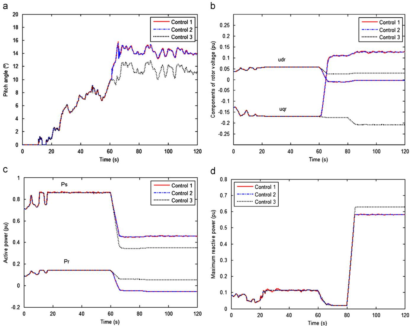
Fig. 16. Comparison of the wind turbine control systems through the response of the wind turbine 3 when the wind farm operates as a PQ node: (a) pitch angle, (b) direct and quadrature components of the rotor voltage, (c) stator and rotor active powers and (d) maximum reactive power.
