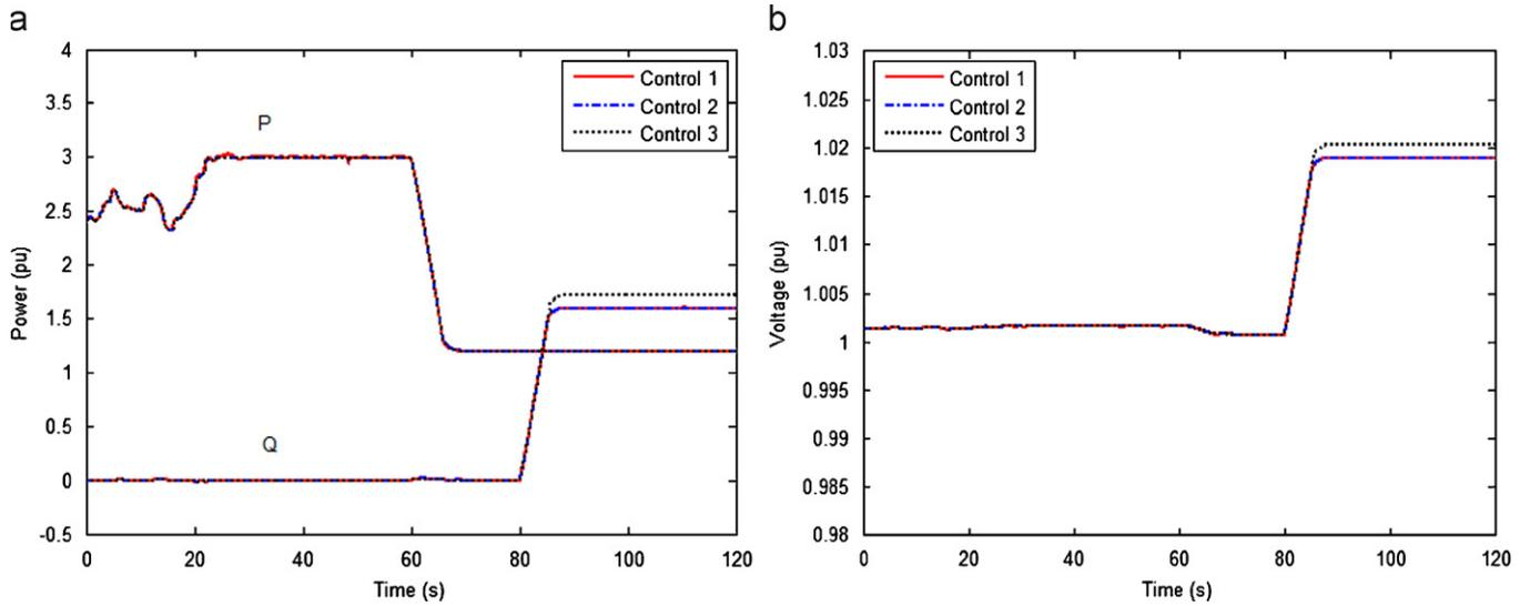
Fig. 14. Response of the wind farm operating as a PQ node: (a) Active and reactive powers and (b) voltage at wind farm node.
