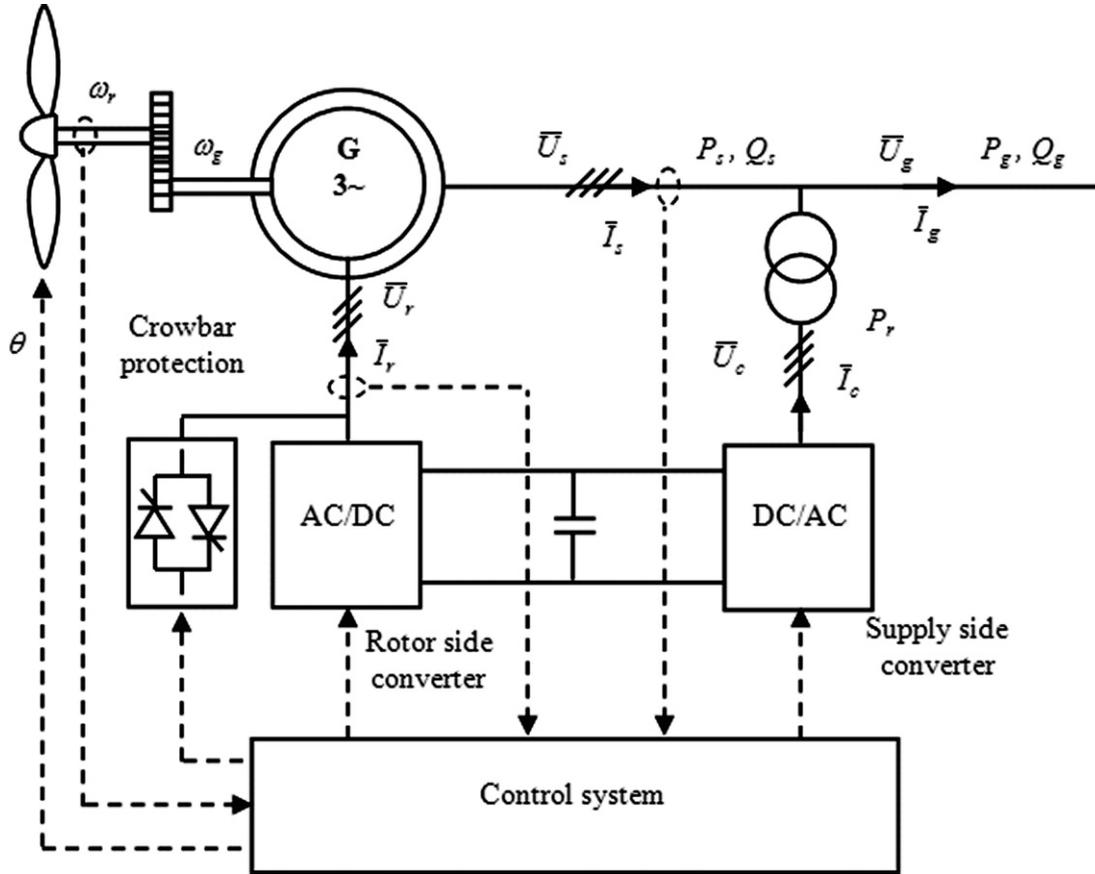
Fig. 1. DFIG wind turbine configuration.
