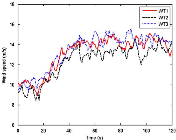
Fig. 13. Wind incident on the wind turbines.
