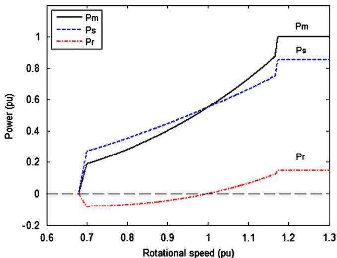
Fig. 4. Mechanical, stator and rotor powers versus rotational speed.
