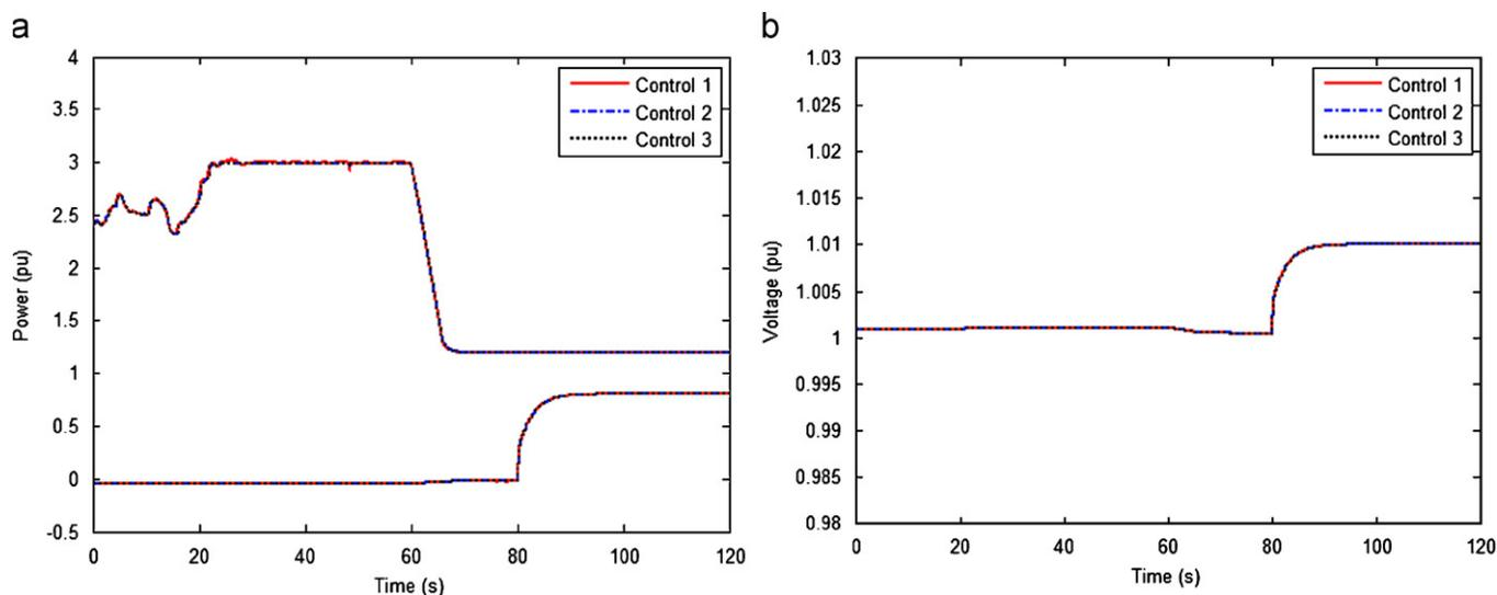
Fig. 17. Response of the wind farm operating as a PV node: (a) active and reactive powers and (b) voltage at wind farm node.
