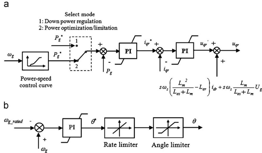
Fig. 9. Control system 3 for DFIG wind turbine: (a)  $u_{qr}$  controller (active power controller with a select mode) and (b) pitch angle controller (speed limiter).
