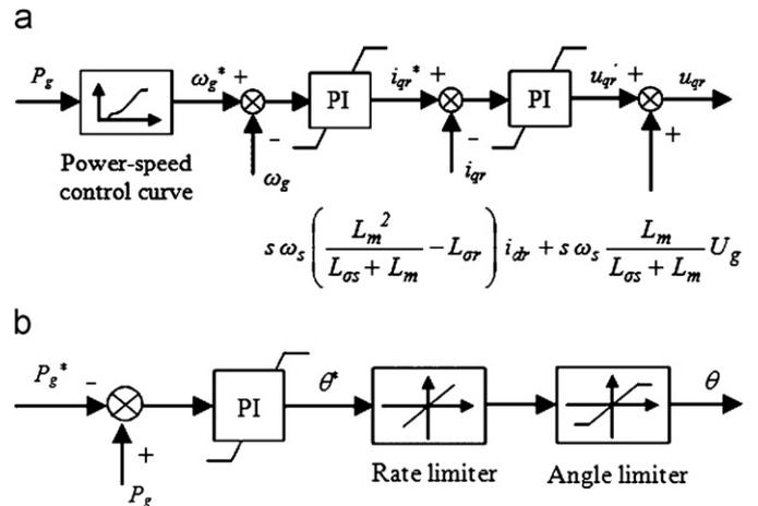
Fig. 7. Control system 1 for DFIG wind turbine: (a)  $u_{qr}$  controller (speed controller) and (b) pitch angle controller (active power controller).
