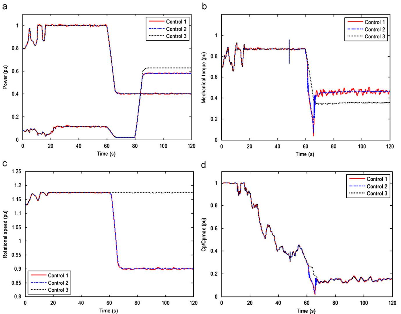
Fig. 15. Comparison of the wind turbine control systems through the response of the wind turbine 3 when the wind farm operates as a PQ node: (a) active and reactive powers, (b) mechanical torque, (c) rotational speed and (d)  $C_p/C_{p,max}$  relation.
